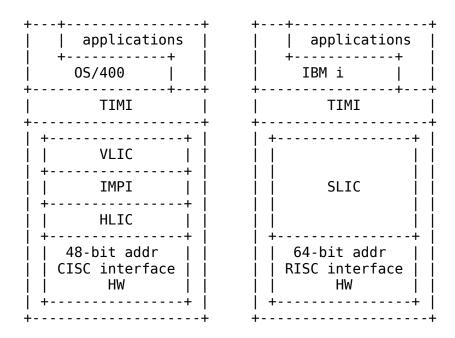
Since the S/38, the system's instruction set defines all pointers as 128-bit. Today, 128-bit processors are already used for special purpose gaming and graphics applications. When at a point in the future 128-bit general purpose processors would appear, IBM i will already be fully 128-bit enabled.
