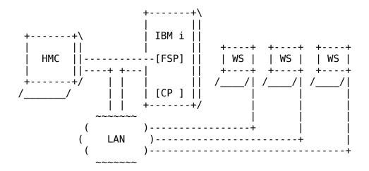
The HMC can be used to initiate the system's Initial Program Load (IPL). Or, simply stated, boot the system. The FSP sends the IPL values to the HMC. For example, code C6004056 means that "Journal recovery is running". You can look up the IPL values of the last boot by using the command "CALL QWCCRTEC". This generates a QPSRVDMP spoolfile.
