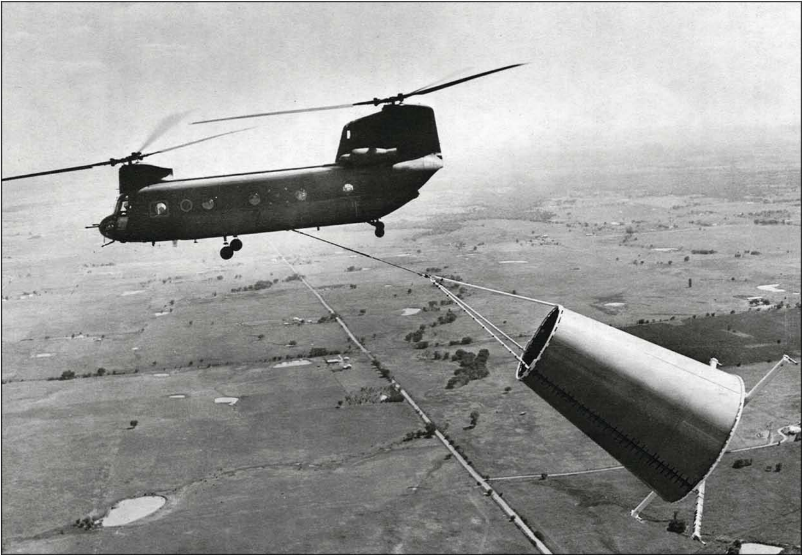
Figure 9-7.- Helicopter transportation of spacecraft/lunar module adapter .
