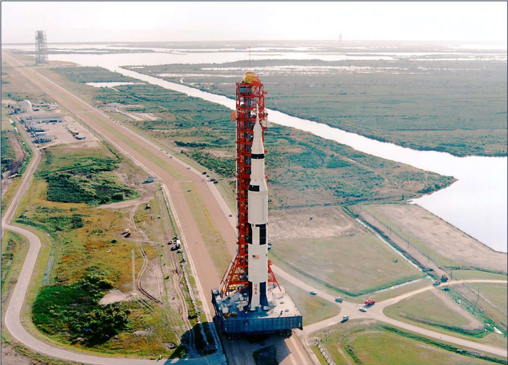
Figure 2-12.- Space vehicle for Apollo 8 mission being transported to Launch Complex 39A.
