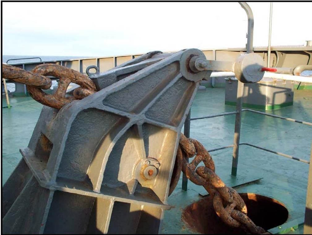
*Fig. 14. The pawl, “guillotine stopper” form the integral part of the anchor cable restraining equipment and is designed to take the anchoring load.*
