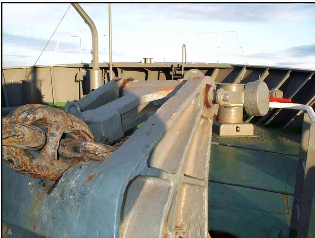
*Fig. 15. Once the required amount of cable has been paid out, the vessel should be allowed to bring-up on the bow stopper.
