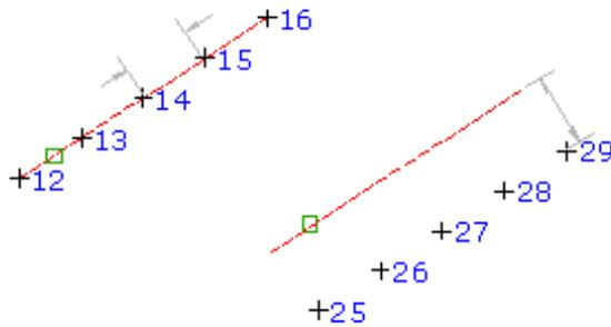
When you create points using this command, you work with one object at a time. After points have been added using a selected object, you can select another object and add points using that object. If the objects you select and the options you specify while using the command would result in the creation of duplicate points, for example, at the shared endpoints of two lines, only a single point is added. Duplicate points are not created.
