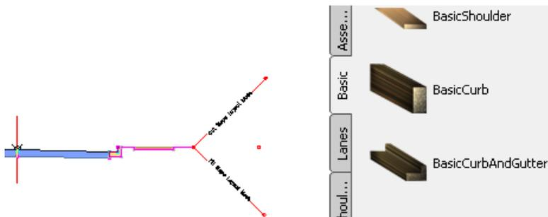
Roadway assembly (left), with subassemblies shown in a tool palette (right)
