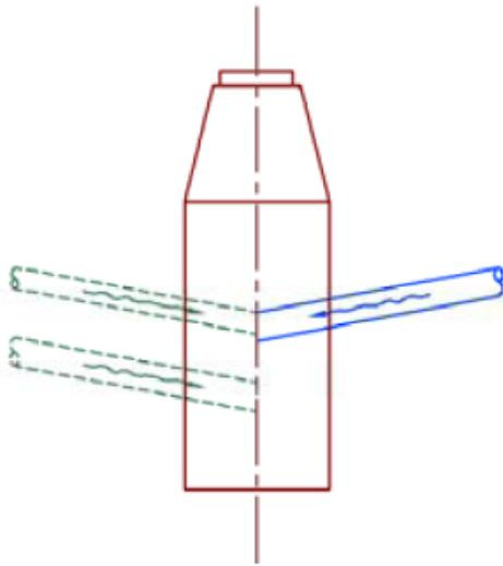
In the following illustration, the junction structure has two incoming pipes already connected to it on the left side of the structure. A new outgoing pipe is added to the right side of the structure. The pipe cover and slope rule determines the optimal connection elevation for the new outgoing pipe.
