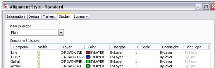
The component layers, such as C-ROAD-LINE, allow you to work with objects as if parts of them are located on different layers. For example, to turn off only the alignment lines, you can turn off the C-ROAD-LINE layer in the drawing.
