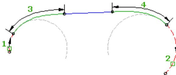
To add a free compound spiral-line-spiral (between two curves, spiral lengths)
