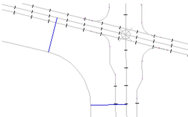
This command calculates the 2D distance between entities. Elevations are not considered in the calculations.
