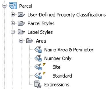
Each label type has a Standard label style. The AutoCAD Civil 3D drawing templates also contain several other label styles you can use.
