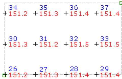
Because this command creates points using elevations from a surface, the Prompt For Elevations setting, specified in the Points Creation settings, does not affect how you are prompted during this command.
