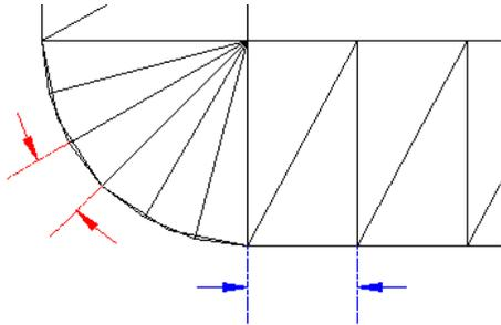
Finer values of spacing lead to a more accurate representation of the grading model, but increase the computation time. These values should be set according to the size of grading object in consideration.
