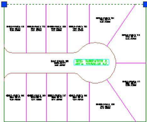
However, the left side of the parcel group is broken up into three segments, as shown below. The span label will not label all three. If you want to label the overall distance of that side, you would need to redraw the left side as one parcel entity.
