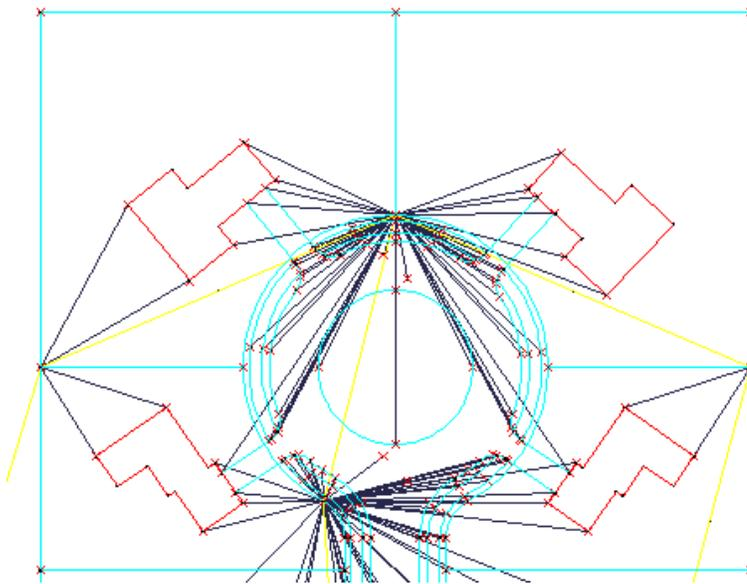
**Linework created by importing survey data using linework coding**
