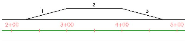
Each [widening](#) (page 2787) includes transition regions at the entry and the exit. In the figure, region 1 is the *entry transition*, and region 3 is the *exit transition*, based on the direction of the centerline alignment. Default values for the length and shape of these transitions are determined by command settings for the AddWidening command.
