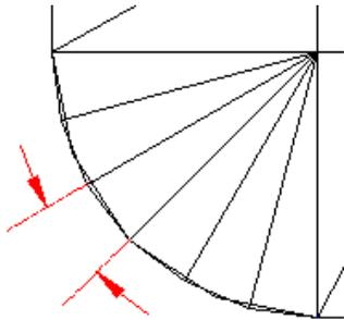
**tessellation spacing** Controls the spacing of supplemental breaklines that are added to a grading along straight segments. Used for surface creation from grading objects.
