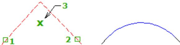
**To create a curve between existing lines through a specified point**
