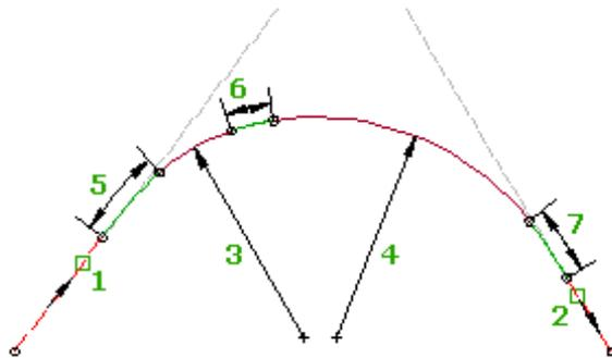
The compound Spiral-Curve-Spiral-Curve-Spiral (SCSCS) group is placed between two tangents. This group is similar to the spiral-curve-spiral (SCS) group, but it has a second curve and spiral at the end of the group.
