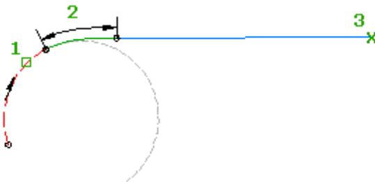
**To add a floating line with a spiral (from curve, through point)**
