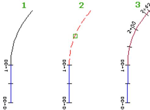
This command is useful when you must add an AutoCAD line or arc onto an existing alignment. AutoCAD lines and arcs can be created using the best fit entities or other lines and curves commands. See [Lines and Curves](#) (page 605) for more information.
