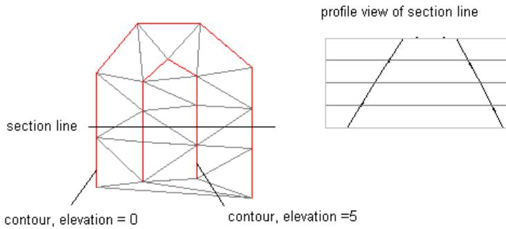
If you run the Minimize Flat Areas operation with the Adding Points to Flat Triangle Edges option, the following results are obtained:
