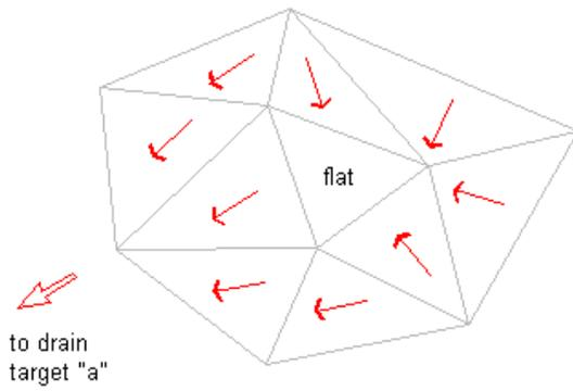
In the following illustration, the flat area, plus whatever part of the surface flows down to it, becomes a flat area watershed. This watershed is ambiguous because water flowing through it can flow to more than one drain target, "a" and "b":
