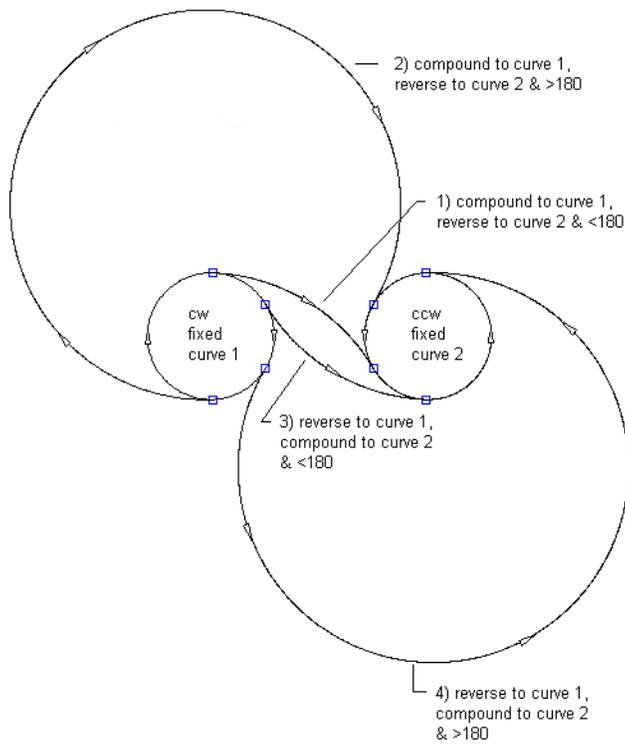
The following illustration shows a free curve fillet between an overlapping clockwise curve and a counter-clockwise curve:
