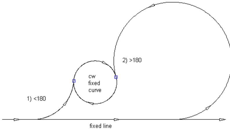
The following illustration shows a free curve fillet between a line and a counter-clockwise curve (on the left) with a specified radius:
