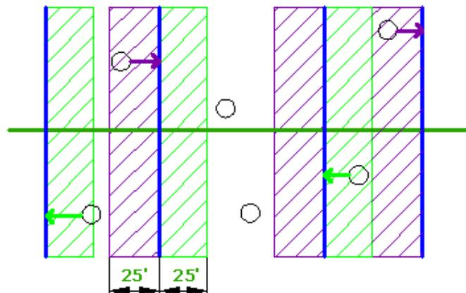
If an object's insertion point is within the area, then it is projected even if part of the object extends beyond the region, as shown by the object in the lower-left corner of the illustration.
