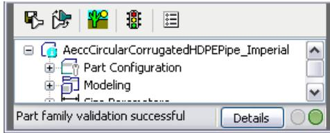
If you have errors in your model, the status bar message displays that the part validation failed, and a dialog box is displayed listing the errors. Review the errors, make necessary modifications, and repeat this step until validation is successful.
