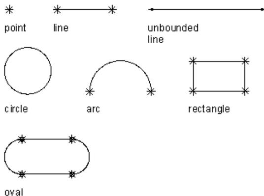
Part Builder provides nine types of geometry you can use to build the model:
