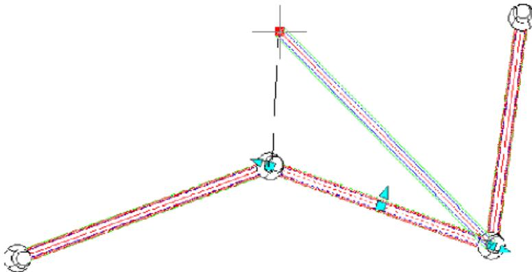
Grip editing a pipe that is connected to a structure does not move the structure along with it. Depending on the rim and sump behaviors of the structure, it may be necessary to adjust the structure vertically to accommodate a new sump elevation, or top of barrel, when the pipe is disconnected from the structure.
