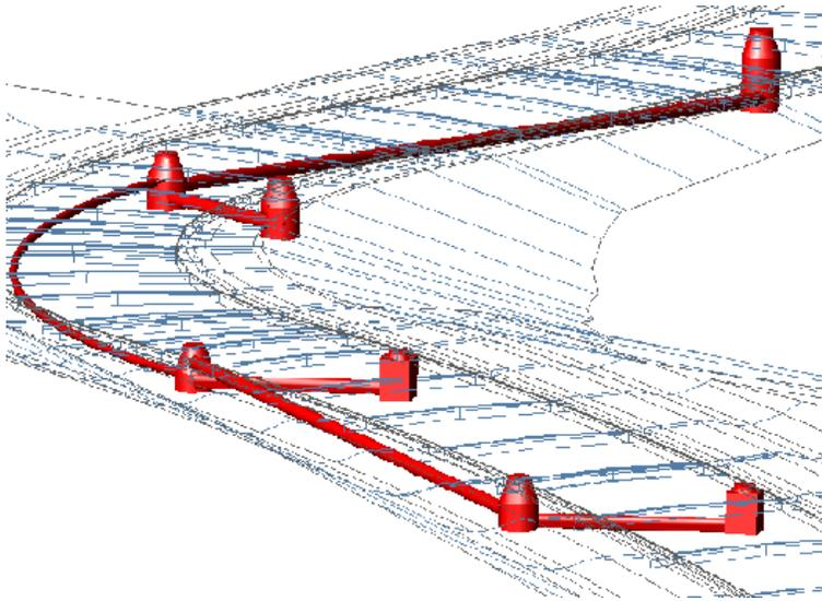
A pipe network can contain pipes only, structures only, or, more commonly, both pipes and structures. A part catalog provides access to pipe network items, such as circular, elliptical, or rectangular pipes, manholes, catch basins, and headwalls, and more.
