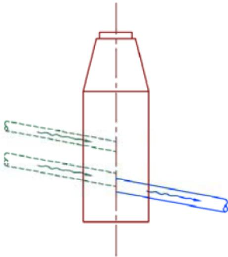
The following illustration shows a junction structure that has two outgoing pipes already connected to it on the left side of the structure. A new incoming pipe is added to the right side of the structure. The pipe cover and slope rule determines the optimal connection elevation for the new incoming pipe.
