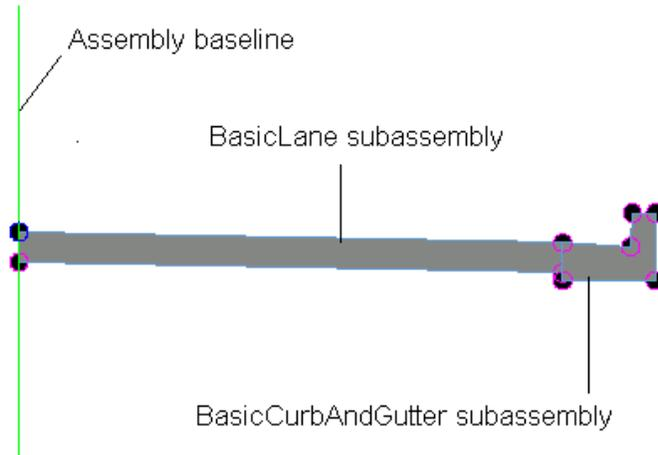
Each subassembly has a defined cross-section, and some subassemblies automatically adapt to their location. For example, the slope of a road lane changes as superelevation is applied, and a side slope automatically creates either a cut or fill slope, depending on the relative elevation of the existing surface.
