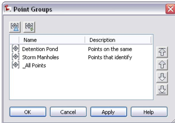
The point group display order for a drawing determines the order in which the point groups are drawn when a drawing is opened or graphics are regenerated. The first (highest) point group in the list is drawn last.
