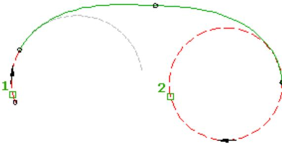
The spiral radii are identical at the spiral-spiral intersection point. The radius value is determined by the total deflection angle and the two spiral lengths. The radius value cannot be edited.
