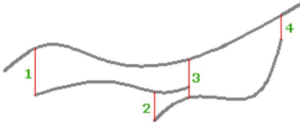
Then the subcriteria are applied as follows, where (1) is subcriteria 1 (below EG, above subsoil), and (2) is subcriteria 2 (below EG, above Rockbed).
