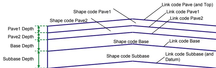
The standard link codes from top to bottom are Pave, Pave1, Pave2, Base, and Subbase. The code Top is also assigned to all finish grade links, thus coinciding with the Pave links on paved sections. The code Datum is also assigned to the bottom of subbase. The shape codes for the material areas from top to bottom are Pave1, Pave2, Base, and Subbase.
