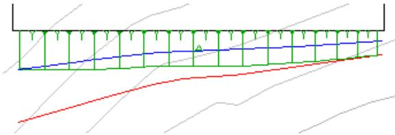
In addition, you are sometimes prompted to create transitions when you use the Create Grading command. This occurs when the start point of a new grading is inside or touching an existing grading.
