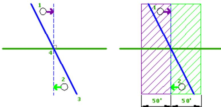
The opposite is true for object 2. It is determined to be after the sample line according to its station, so the rules for “after” are applied to it. Since both objects fall into either a “before” or “after” region, they are both projected.
