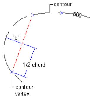
if ratio of "d" to 1/2 chord  $>$  supplementing bulge factor, then vertices will be added on the arc
