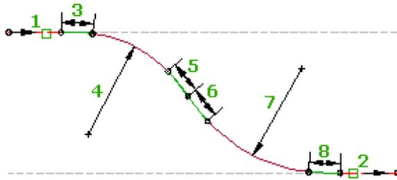
You cannot grip edit the reverse SCSSCS group, but you can edit the tangents to which it is attached. You can edit the spiral or curve parameters directly in either the [Alignment Layout Parameters](#) (page 1953) dialog box or the [Alignment Entities](#) (page 1947) vista.
