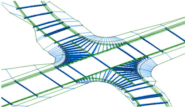
Another approach to creating intersections is to first create roadway alignments, offset alignments, and profiles. Once these preliminary design items are in place, you can create an intersection object that utilizes the 3D aspects of these road design geometry components.
