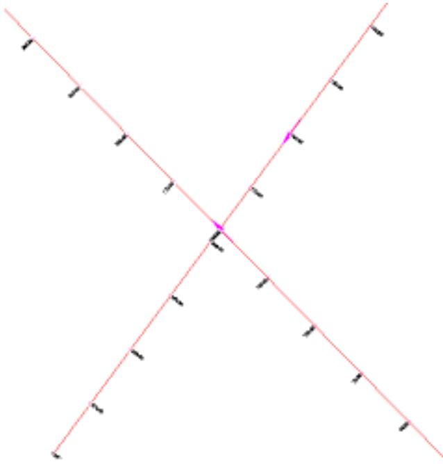
In this example, the two alignments intersect each other, and they both pass through the roundabout location on both sides.
