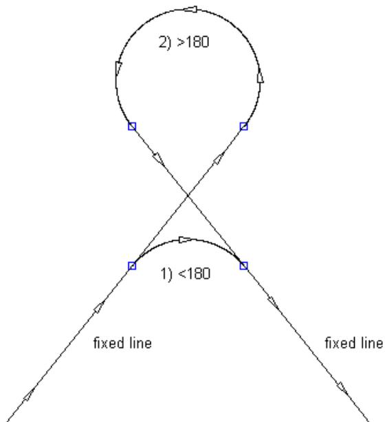
The following illustration shows a free curve fillet between two fixed clockwise curves:
