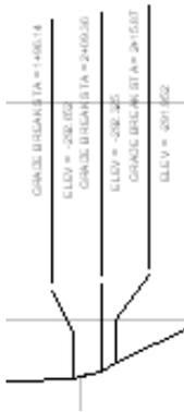
**Profile with staggered labels to avoid collisions**
