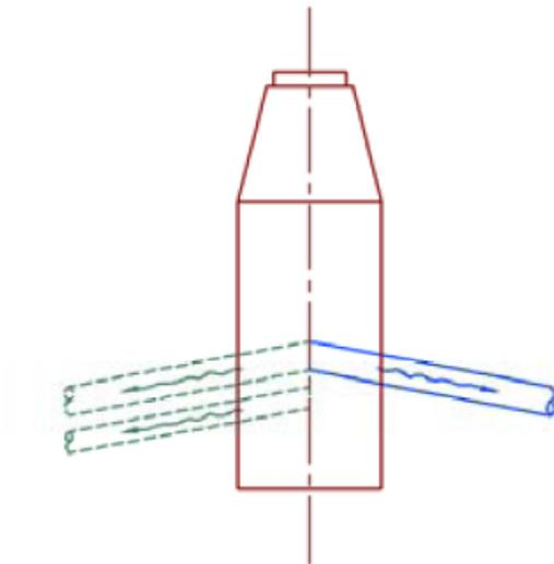
The following illustration shows a junction structure that has four pipes already connected to it on the left side of the structure. Two of those pipes are incoming pipes, and the other two are outgoing pipes. A new *incoming* pipe is added to the right side of the structure. The pipe cover and slope rule determines the optimal connection elevation for the new incoming pipe.
