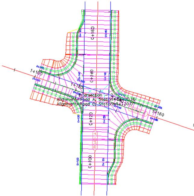
Before creating an intersection object, you must have two alignments that intersect. If you want to create a three-dimensional intersection model, you must also have profiles associated with the intersecting alignments. Once you have the desired prerequisites, then you can create the intersection object using the Create Intersection wizard.
