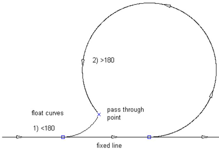
The following illustration shows a floating compound curve attached to a curve and four possible solutions for a given radius and pass-through point. The illustration also shows variables for greater than and less than 180 degrees and compound and reverse variables:
