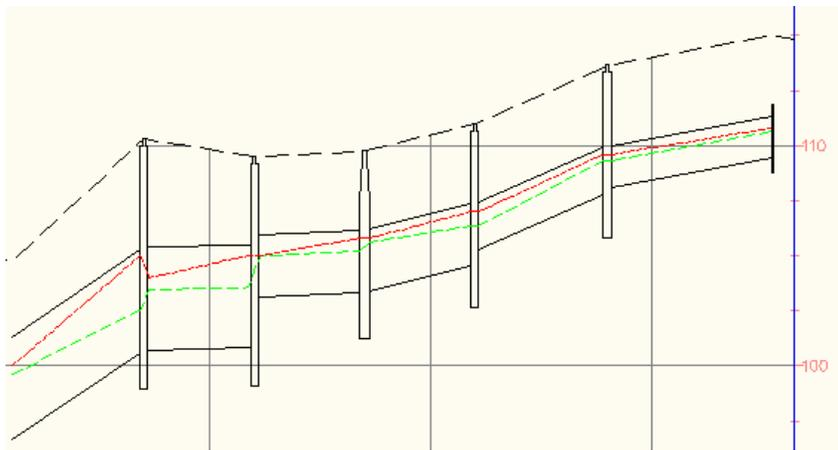
The energy grade line is displayed as a red dashed lined (on the top). The hydraulic grade line is displayed as a green dashed line (below the energy grade line).
