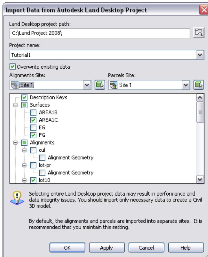
The recommended use of this Import function is to bring individual surfaces, alignments, or pipe runs into new drawings for use in AutoCAD Civil 3D projects.
