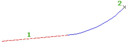
**To add a fixed vertical curve with an entity and a pass-through point**
