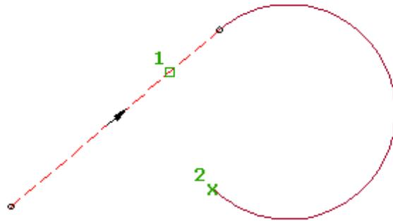
The result is a floating curve that is always tangent to the entity it is attached to.
