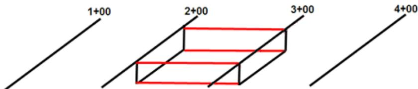
If marsh material is present between station 2+00 and 3+00 with short transitions before and after, you can specify run in and run out instead of adding more sample lines, as shown in the following illustration.
