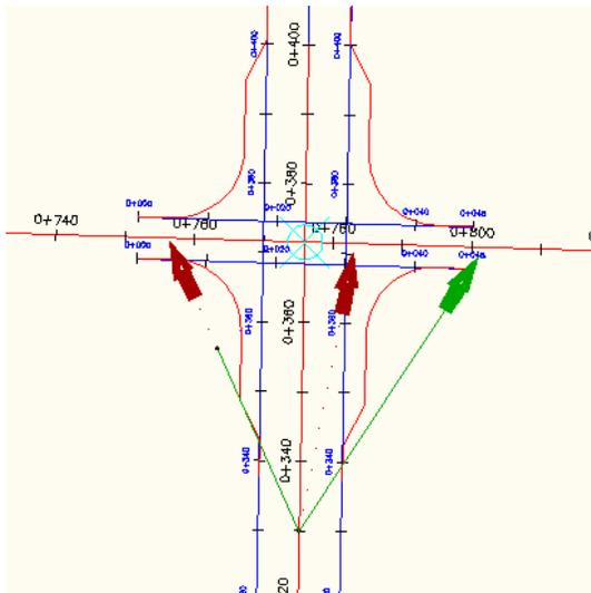
If the target is not visible from the eye location, the portion of the line of sight that is visible is green and the line beyond the obstruction point is red. A message is displayed at the command line indicating that the line of sight is obstructed. The name of the surface that is causing the obstruction, the obstruction point coordinates, and the distance from the eye to the target are listed.
