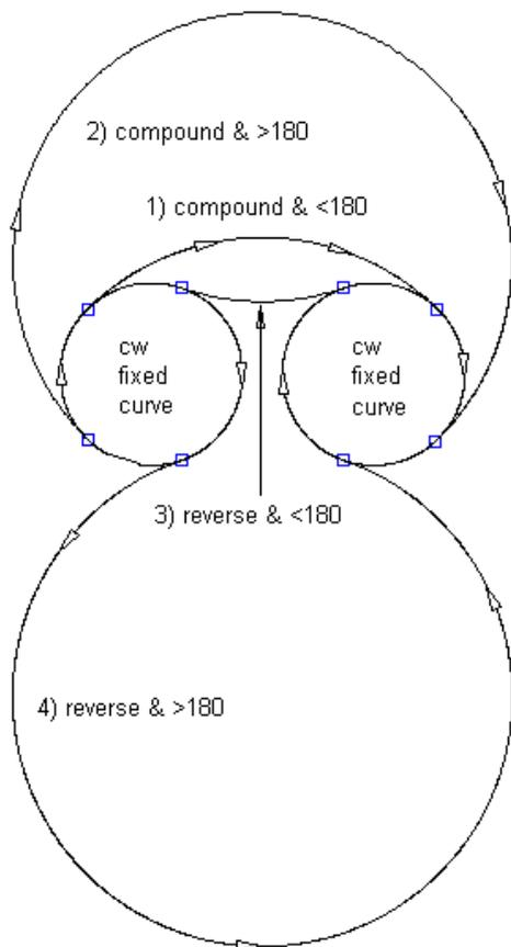
The following illustration shows a free curve fillet between a fixed clockwise curve and a fixed counter-clockwise curve:
