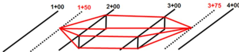
The run in for the material is defined in the first gap, and the run out for the material is defined in the second gap. Therefore, the first gap would have a run in of 50, and the second gap would have a run out of 75.
