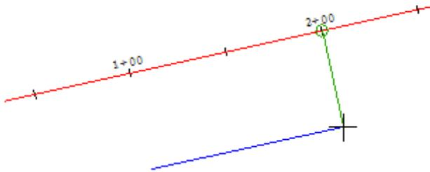
**To create a line by specifying station and offset from an alignment**
