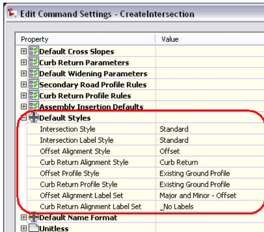
You can also create label sets for offset alignments and for curb return alignments.
