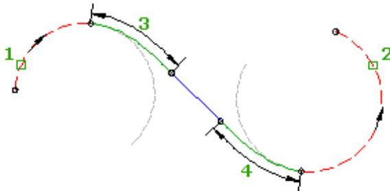
In this command you can specify the spiral parameters, but not the line length. Line length is calculated automatically.
