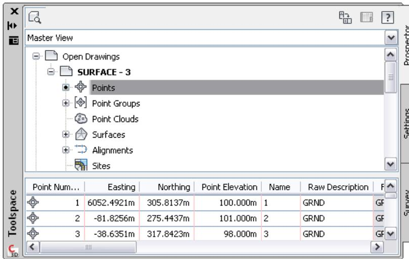
When the Toolspace is docked, the list view is displayed below the data tree. When the Toolspace is undocked, you can display the item view either below the data tree or to one side of the data tree by clicking the item view orientation button
