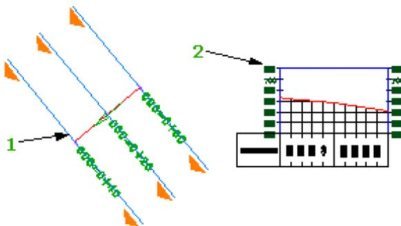
Each section view must be linked to an alignment. The section view displays new or existing sections. Sections can also be created without displaying them on a section view. When you create a section view for an alignment, the complete list of sections for the alignment is displayed. Choose which sections to include in the section view.
