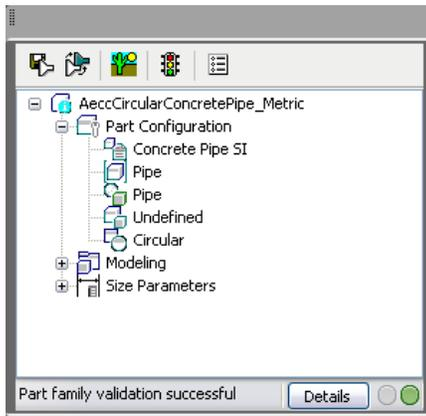
The part configuration is defined once for a part family and remains constant for all part sizes. The following components are required to define the part configuration:
