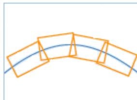
The view frames will be aligned along the alignment. Typically, this is the preferred method for making the most efficient use of paper when plotting.
