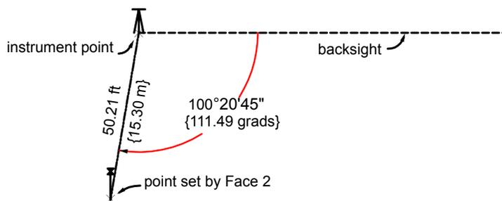
Point 101 is located a distance of 15.30 from the instrument setup at an observed angle right from the backsight of 311.4954. The actual physical angle turned is 111.49, with a vertical angle of 301.03. The description for the point is IP. Angles and distances are in the current units, unless you type a qualifying suffix.
