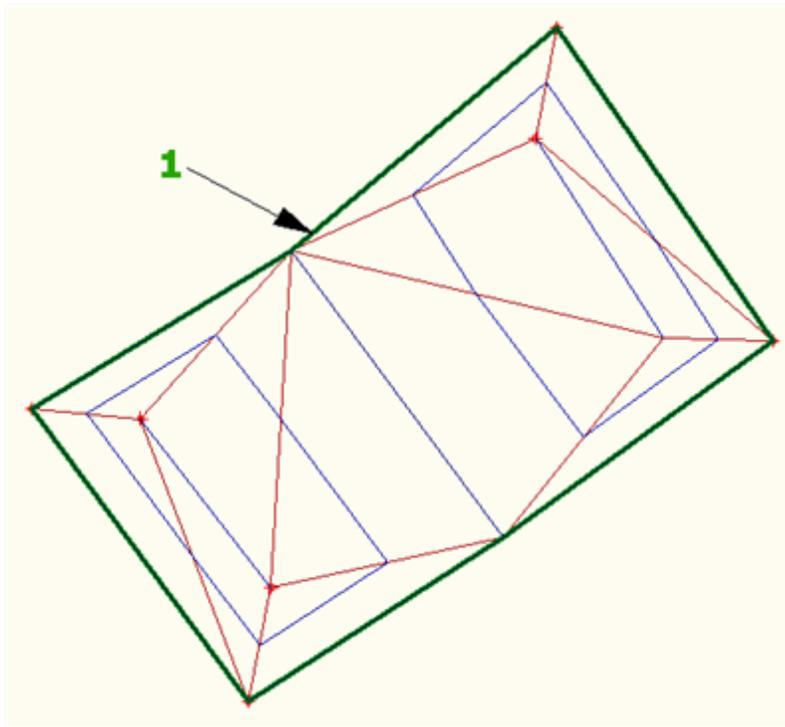
The surface object data is extracted, and listed in the Stage Storage Volume Table. This option uses all the contour data from the surface.
