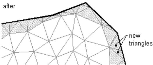
If you create a boundary without non-destructive breaklines along the boundary edges, only triangles that are completely within or outside the boundary are affected:
