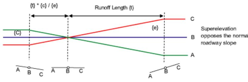
In the following example, the Continuing section defines the Normal Crown to Full Superlevation distance runoff length  $\{t\}$  (derived from the transition length tables), minus the runoff length times the normal roadway slope  $\{c\}$  divided by the full superlevation rate  $\{e\}$ . The second formula defines the distance from Normal Crown to the Beginning of Curve as a percentage of  $\{t\}$  based on the variable  $\{p\}$  minus  $\{c\}$  divided by  $\{e\}$ .
