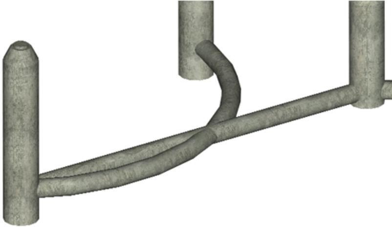
If desired, you can also perform a check for pipe network parts in their 3D representation that are too close to one another, according to predefined distance or scale factor criteria. In the following illustration, the two pipe networks shown are less than ten feet away from each other at the closest point, even though they do not physically collide:
