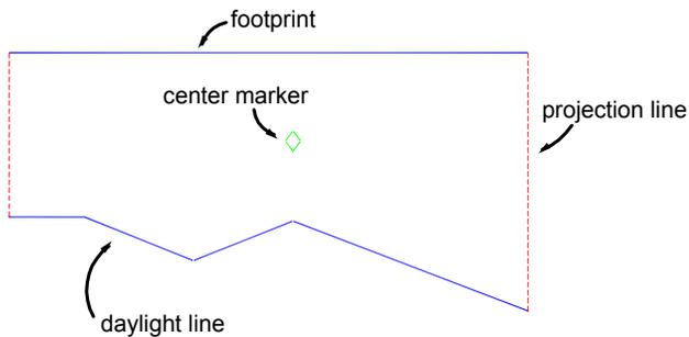
The footprint can be an open or closed figure. The footprint must be either a [feature line](#) (page 2774), a lot line, or the resulting [daylight line](#) (page 2772) of another grading.
