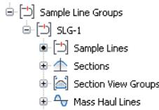
If one or more sample line groups have been added to the current drawing, expand the Sample Line Groups collection to view the names of the sample line groups. A tabular list of the sample line groups is displayed in the item view at the bottom of the Prospector tab.
