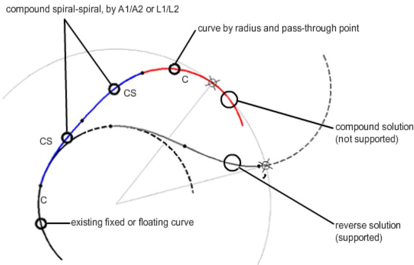
**To add a floating reverse curve with spirals (from curve, radius, through point) off a curve**
