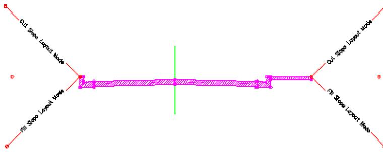
An assembly object, like its corridor and subassembly counterparts, can adapt to conditions such as superelevation and cut or fill requirements.
