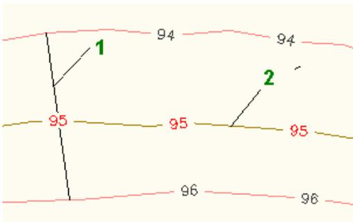
Modify the properties of contour label lines to change the label style for major, minor, and user-defined contour labels.
