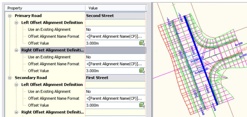
The right side offset alignment named First Street is selected in the Intersection Offset parameters dialog box, shown on the left. In the drawing, that offset alignment is highlighted.
