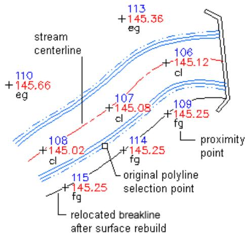
Define proximity breaklines by selecting a polyline. You do not have to draw the polyline precisely between surface points. The breakline definition automatically snaps to the surface point that is nearest each polyline vertex when the breakline is added to the surface.
