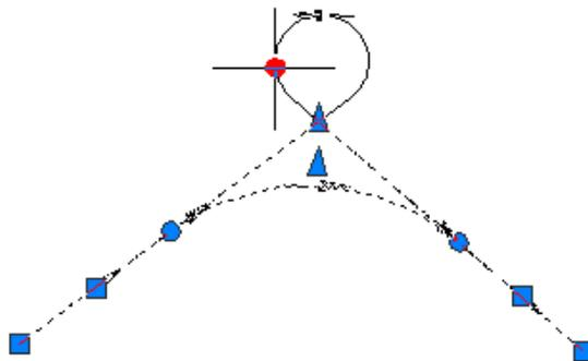
Changing the radius to greater than 180 degrees using the triangular radius grip:
