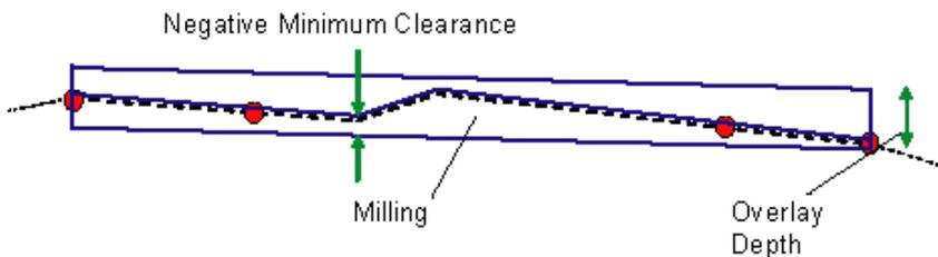
The milling report identifies the begin and end stations where milling occurs; left and right offsets from the centerline at the begin and end stations; and the area that is calculated from the previous data.
