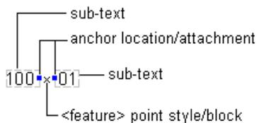
The following examples illustrate a label style that can label a spot elevation at the elevation decimal point. The decimal point of the spot elevation value is represented by a block, or a point style specified at creation time. The labeled elevation consists of two subtext components in the label style, each with different properties:
