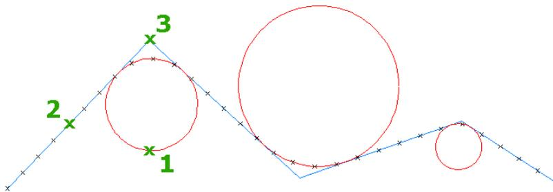
When the Create Spirals option is selected, AutoCAD Civil 3D creates a symmetrical pair of spirals (1) between each curve and its tangents. If spirals that meet the specified R/A value do not fit between the tangents (2) and the curve (3), then the curve radius is reduced (4) until a solution is found. When you specify this option without the Match Tangents option, the spirals will be symmetrical, but the solution may have greater error.
