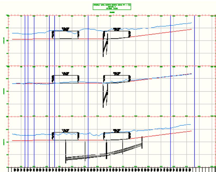
A profile can be split within either a single or multiple profile view. This allows a profile view to display a profile elevation range that is greater than the specified height of the profile view.
