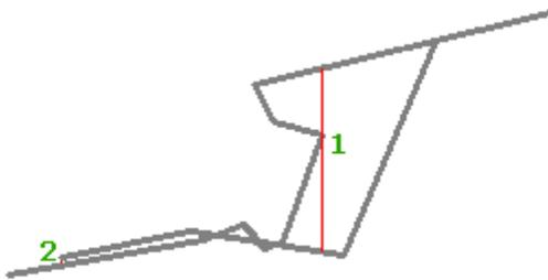
Then the subcriteria are applied as follows, where (1) is subcriteria 1 (above Datum, below Rock Bed), (2) is subcriteria 2 (above Rock Under, below Rock Top), and (3) is subcriteria 3 (above Datum, below Rock Top).
