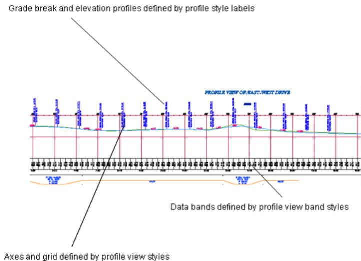
Profile view displaying surface and layout profiles
