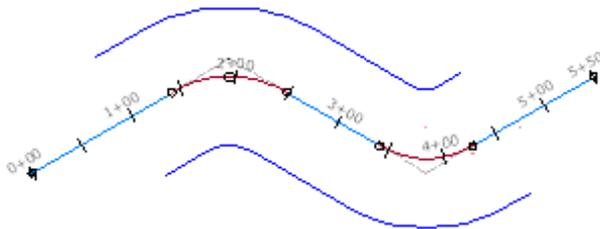
Left and right sides are determined from a position facing toward the end of the parent alignment.
