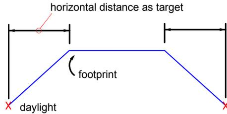
Section view of distance as target
