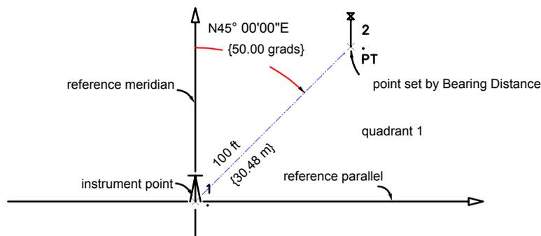
Point 2 is located by turning a bearing of 45°0'0" (50 grads) in Quadrant 1 (NE) at a distance of 100 feet from the instrument point with the description PT.
