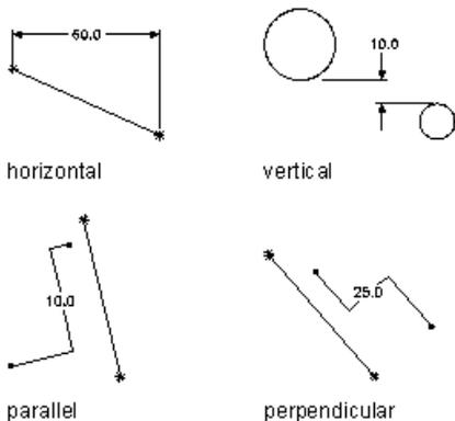
Part Builder provides seven types of dimensions you can add to the model:
