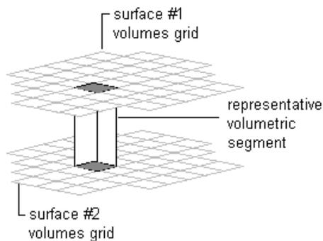
A grid volume surface is an approximation of the difference between the base and comparison surfaces. It is formed by making a grid from points whose Z values are the differences between the Z values of the comparison and base surfaces. Therefore, the grid volume surface gives the exact difference only at the grid points. This is true whether the comparison and base surfaces are both grid surfaces, both TIN surfaces, or one of each.
