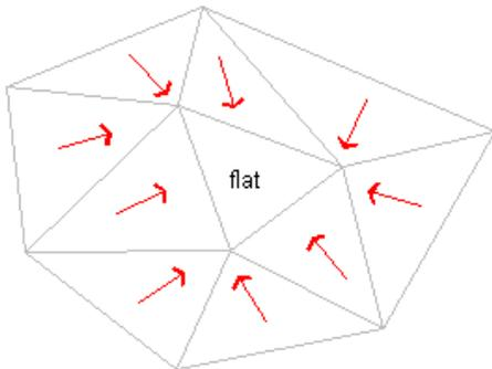
If some of the opposing, non-flat triangles slope down from the flat area boundary, but all flow to the same drain target "a", as shown in the following illustration:
