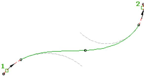
By default, the two spirals have equal lengths and A values. Both values can be modified at the time of creation by specifying a ratio of  $A1/A2$  or  $L1/L2$ .
