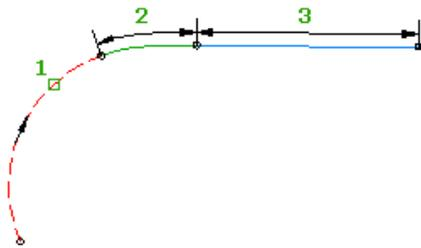
To add a floating line with spiral (from curve end, length)
