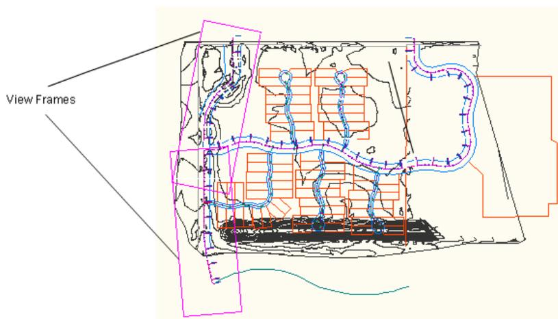
**View frames represent the alignment data that will be displayed in layout sheets**
