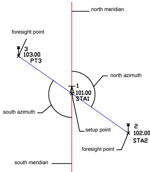
**backsight** A previously established point used as a direction reference to another point. A survey instrument movements typically are locked to an angle of 0 degrees, and the vertical crosshair is set on the backsight. All subsequent shots are then taken by turning the instrument and the upper movement together, while the lower movement stays set on the backsight. All angles measured are, therefore, relative to the backsight.
