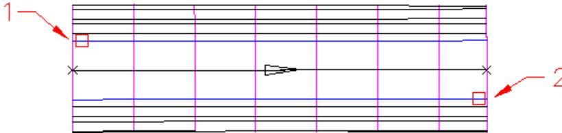
If you are creating the corridor boundary using a polygon, you can create the required polygon by exporting corridor feature lines as polylines, and then join them to create the required polygon.
