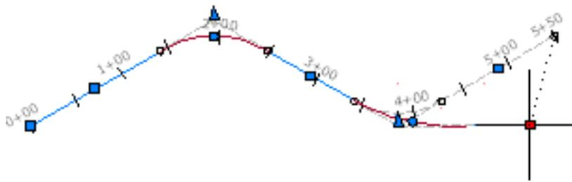
You use the Alignment Layout Tools toolbar, Alignment Layout Parameters dialog box, and Alignment Entities vista to edit an alignment. These dialog boxes remain open if you either grip edit or deselect the alignment, or enter another command.
