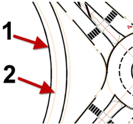
The first arrow (1) identifies the road marking solid line (polyline). The second arrow (2) identifies the slip lane alignment for the left edge of the slip lane.
