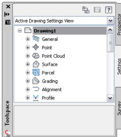
On this tab, styles are organized for different object types. Even in a blank drawing, most of these styles are present in a standard hierarchy. You can create and modify styles in a drawing, then save it as a template. Subsequent drawings based on the template will automatically have the same set of styles available. You can modify object, label, and table styles. You can also control settings for drawings and commands.
