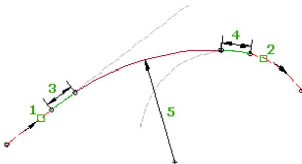
The Spiral-Curve-Spiral command is similar to the command that adds a free curve by radius between two entities. However, this command adds a transition spiral in and a transition spiral out. The curve group for
