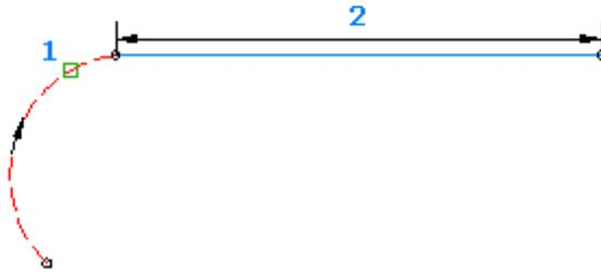
The line is tangent to the end of the selected fixed or floating entity when it is created. If you edit the line or the entity it is attached to, tangency is not maintained.
