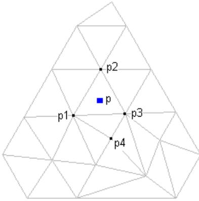
Using NNI, you select only the output locations of the interpolated points. The elevations of the interpolated points are always based on the weighted average of the elevations of the existing neighboring points. The outcome of the NNI method is more predictable than the Kriging method. NNI interpolates only within the surface, whereas Kriging can extrapolate beyond the surface border based on a selected polygon.
