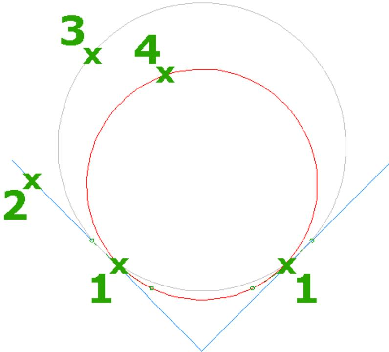
When the Match Tangents option is selected, AutoCAD Civil 3D creates an asymmetrical pair of spirals (1, 2) between each curve (3) and its tangents (4, 5). If a spiral that meets the specified minimum R/A ratio does not fit between a curve and a tangent, then the tangent (4) is moved toward the curve until a solution is found. The minimum R/A value enables you to restrict the spiral lengths; a higher value produces shorter spirals, while a lower value produces longer spirals.
