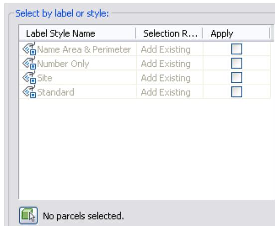
To add all labels of a particular label style name to a table, select the Apply check box next to the label style name. When you use this method, all the labels are switched to tag mode, and a child style is not created.
