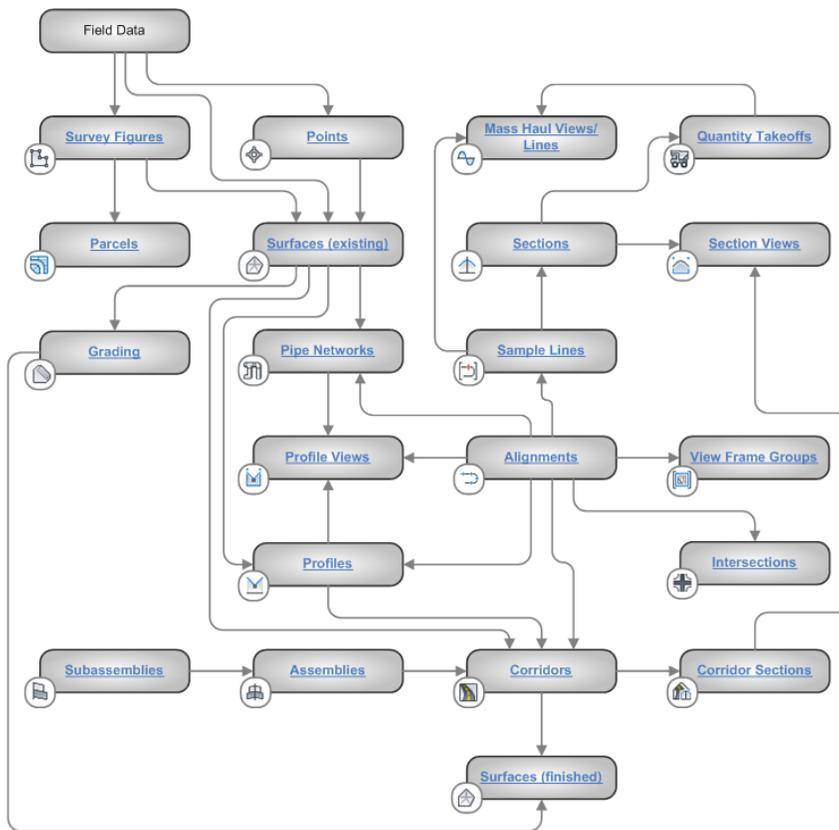
Field data creates a set of points that are used to generate an existing ground surface. This surface is referenced by other objects as indicated by the arrows.
