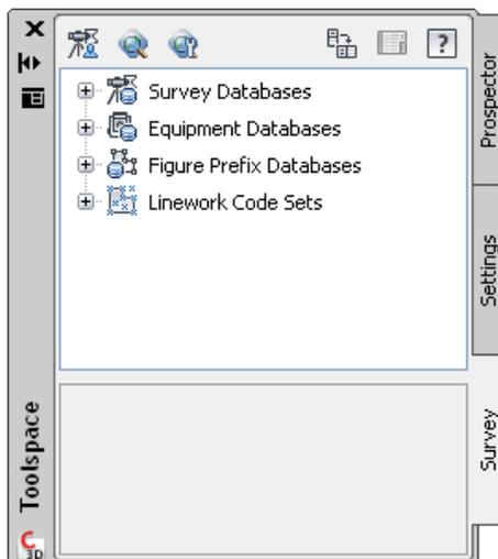
This tab displays survey project data, organized within databases for survey projects, equipment, and figure prefixes. The project databases record the survey points, networks, and figures. The equipment databases record standard deviations and other operational parameters of individual pieces of survey equipment. The figure prefix databases record the conversion routines that are applied when creating lots, buildings, or other figures from survey points.
