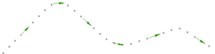
When two paths of roughly parallel COGO points are used, an AutoCAD spline (1, 2) is created through each path of points. The points from each spline are projected onto the other spline; points where the two projections meet are used to create the centerline (3).
