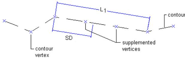
if  $L1 >$  supplementing distance, then vertices are added in equal increments that are less than or equal to SD
