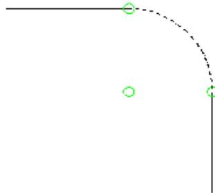
The curve is highlighted and the arc start, center and end points are displayed with glyphs.
