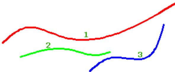
(1) is top of Existing Ground, (2) is top of Subsoil, and (3) is top of Rockbed.
