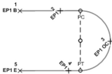
Curve Fit - Three-point curve: In the following illustration, each point has the same EP1 figure name, and there is three consecutive curve points (OC <Point on curve> code, or BC <Begin curve> code at the beginning of the curve). The resulting figure will have a begin curve (BC) at the first EP1 point, an end curve (EC) at the third EP1 point, and the curve will pass through the second EP1 point.
