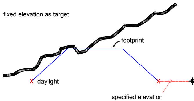
Section view of elevation as target
