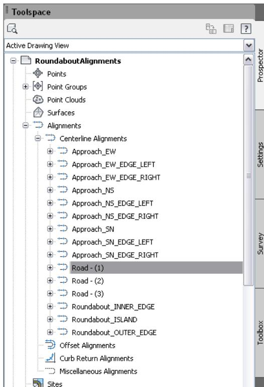
If the selected base alignments are associated with sites, then the resulting roundabout alignments are displayed in the appropriate Sites collection, under Sites ► Alignments ► Centerline Alignments.
