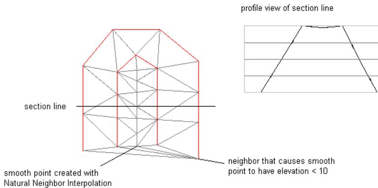
These results occur because the NNI interpolation uses surrounding points to determine an appropriate elevation for a new point. Because all surrounding elevations are lower than the flat triangle, elevations lower than the flat triangle are selected for the added points, resulting in the dip in the ridge.
