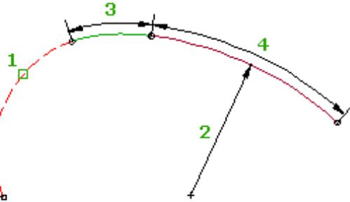
To add a floating curve with a spiral (from entity, radius, length) off a line
