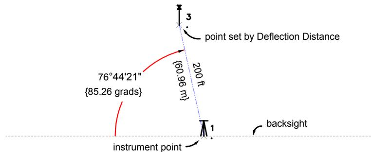
Point 3 is located by turning a deflected angle of 85.2657 right from the extension of the backsight line at a distance of 200. Angles and distances are in the current units, unless you type a qualifying suffix.
