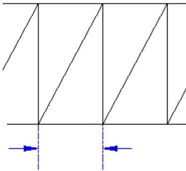
**tick** A component of a label that is usually a mark (or short line) inserted in a series at perpendicular angles to another object, such as a line or curve.
