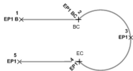
Curve Fit - Multi-point curves: In the following illustration, each point has the same CL1 figure name, and there are more than three consecutive points with an OC <Point on curve> code, or the first point on the curve segments has a BC <Begin curve> code and the ending point of the curve segments has an EC <End curve> code. The resulting figure will have a beginning of curve (BC) at the first CL1 point, and an end of curve (EC)
