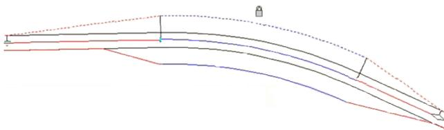
In the command settings for alignment commands, you can configure a variety of options to control default behavior for how widenings and transitions are created in widening situations. For example, on the AddWidening command, you can configure the default settings for how the Linear Transition Around Curves
