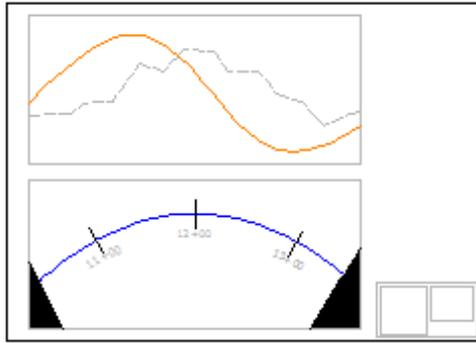
The match line mask area is the area that exists between the outside of a match line and the inside border or boundary of the view frame. On the Display tab of the Match Line Style dialog box, there is an option to set the hatch pattern for this match line mask area.
