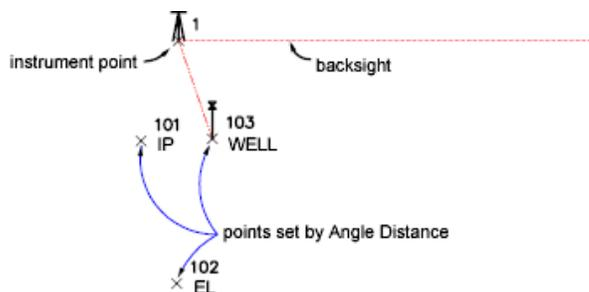
Point 101 is located by turning a horizontal angle of 100°20'45" right from the backsight and using a vertical angle of 91°15'15" at a distance of 100 units from the instrument point with the description IP.
