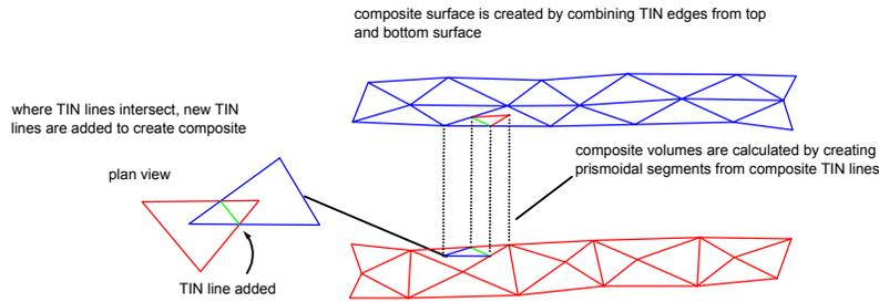
This method gives accurate volume measurements between the two surface definitions.
