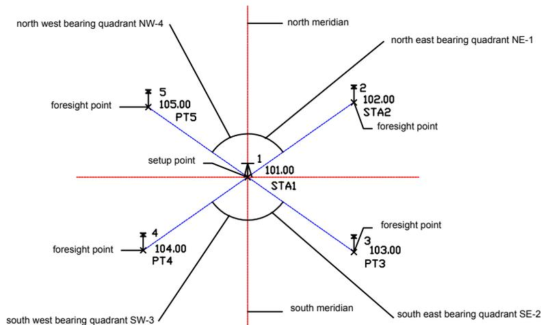
An azimuth is measured clockwise from either the north or south meridian and is always less than or equal to 2PI.
