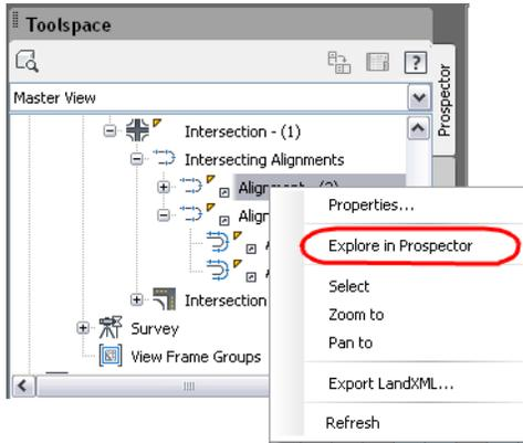
To use this command, right-click an alignment in the Intersecting Alignments collection, and select Explore In Prospector.
