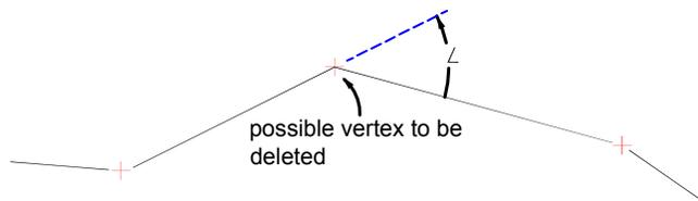
if  $\text{angle} < \text{angle factor}$ , then the vertex will be deleted
