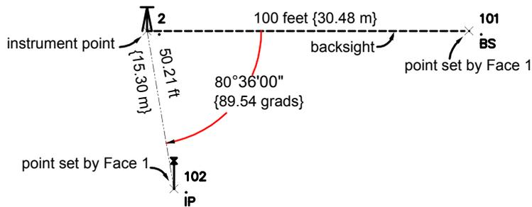
Point 101 is located by turning a horizontal angle of 0 right from Face1, and a vertical angle of 100 at a distance of 30.480 from the instrument point with the description BS.
