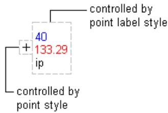
Although an individual point can reference a point style and a point label style, when possible, you will want to use point groups to control the display of point symbols and point labels for points sharing similar characteristics. For more information, see [Controlling the Appearance of Points in a Drawing](#) (page 454).
