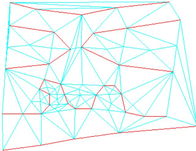
One benefit of the Swapping Edges option is that it does not increase the size of the surface. The Adding Points To Flat Triangle Edges and Adding Points To Flat Edges options generally produce better results, but they increase the size of the surface.
