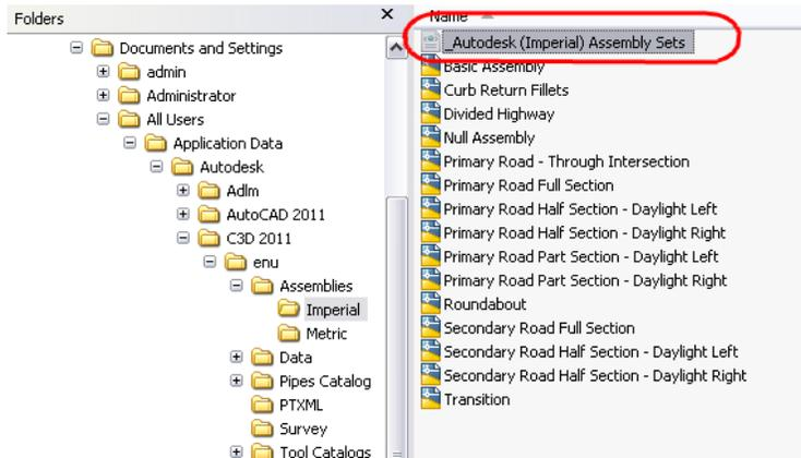
When you apply the assembly set, and create or update the intersection object corridors, the referenced assembly objects are imported into the current drawing, if they are not already there.
