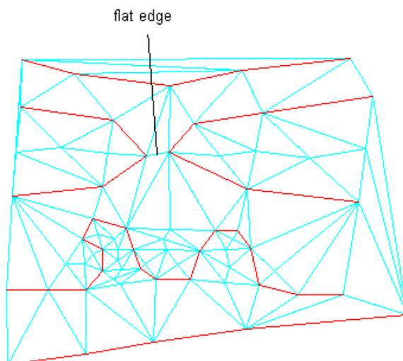
In this illustration, 27 points are added to the surface. Most flat triangles are removed, except for some along the top and upper left borders.
