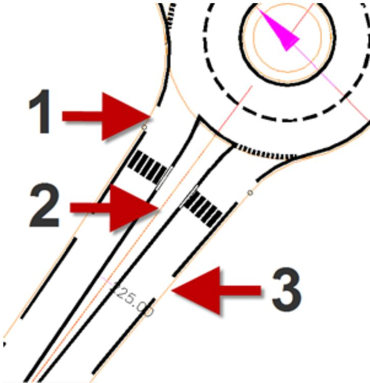
The island, construction triangle, and pavement markings on the approach road are constructed as polylines.
