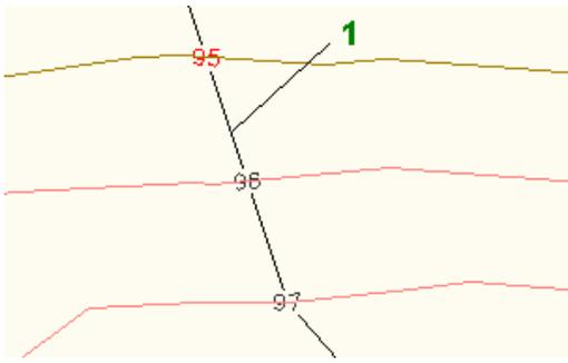
To make a contour label mask out the contour use the Background Mask property in the contour label style. Edit the contour label style using the Label Style Composer, and on the Layout tab under Border, set the value for Background Mask to True.
