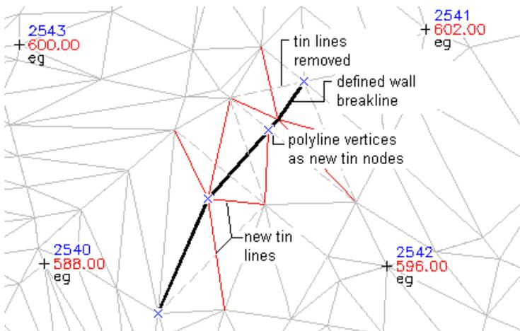
There are two methods used to define wall breaklines:
