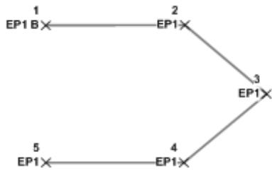
Curve Fit - One point on curve: In the following illustration each point has the same EP1 figure name, and one survey point is coded as a curve point (OC <Point on curve> code). The resulting figure will have a calculated point of curvature (PC) and point of tangency (PT), and the curve will pass through the point.
