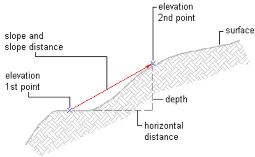
The slope can be labeled as a grade or slope, and is formatted using the slope label style. The direction of the slope is represented by a directional arrow component defined in the slope label style.
