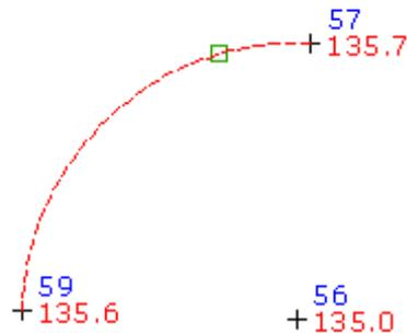
When you create points using this command, you work with one object at a time. After points have been added using a selected object, you can select another object and add points using that object. If the objects you select and the options you specify while using the command would result in the creation of duplicate
