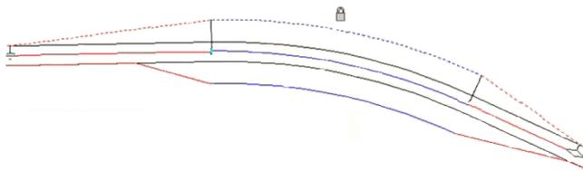
You can control the widening values and transition lengths by specifying properties, such as the number of lanes, vehicle type, wheelbase lengths, design speeds, and so on, in a design criteria file associated with the parent alignment. You can also specify widening values and transition lengths manually by entering values into the Add Automatic Widening dialog box. The automatically widened curves remain dynamic to the parent alignment geometry based on the specified criteria.
