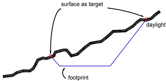
Section view of surface as target
