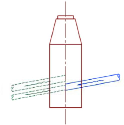
The following illustration shows a junction structure that has two outgoing pipes already connected to it on the left side of the structure. A new outgoing pipe is added to the right side of the structure. The pipe cover and slope rule determines the optimal connection elevation for the new outgoing pipe.
