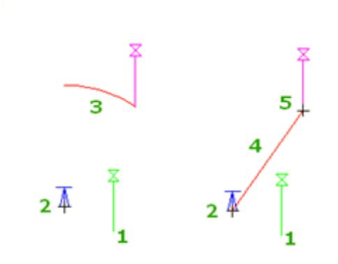
A transparent command can only be used within a running command. The reference line is updated each time you enter a point.
