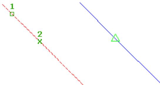
Split points are created when two feature lines cross and neither has a geometry point. A split point cannot be edited as it is controlled by the grades of the two crossing segments which must have the same elevation at the crossing point. If their elevations are different, a grade break will be inserted into one to match the
