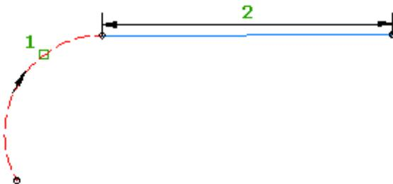
This type of entity always starts at the end of the entity it is attached to. The line is always tangent to the end of a fixed or floating curve. Unlike an entity where the location is defined by a pass-through point, this type of entity is not pinned to a location in the drawing. Therefore, the entity geometry moves with the entity to which it is attached.
