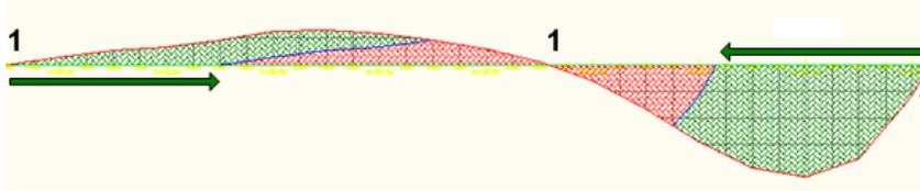
**Balance Point Method:** The arrows indicate free haul distance. The number (1) indicates balance points. Freehaul volume is indicated in green and overhaul volume is indicated in red.
