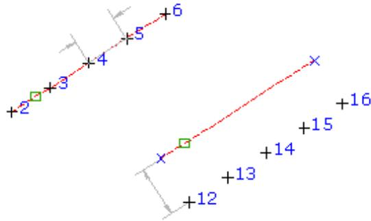
When you create points using this command, you work with one object at a time. After points have been added using a selected object, you can select another object and add points using that object. If the objects you select and the options you specify while using the command would result in the creation of duplicate points, for example, at the shared endpoints of two lines, only a single point is added. Duplicate points are not created.
