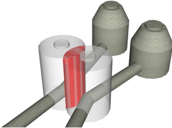
Another type of interference that can be detected is when two pipes intersect without a structure joining them, as shown in the following illustrations:
