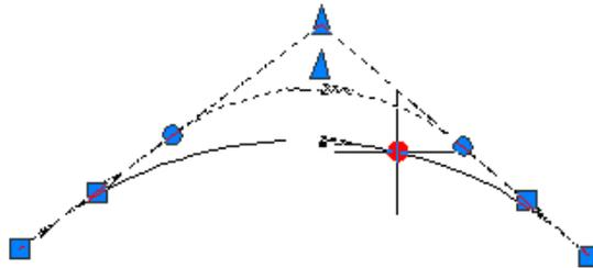
Changing the radius to greater than 180 degrees using the circular pass-through point grip:
