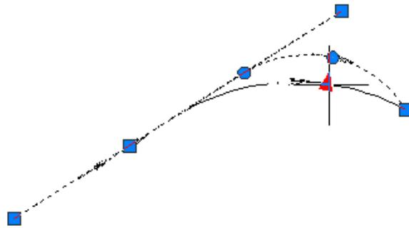
**To use grips to edit a floating curve attached to an entity end with a pass-through point**
