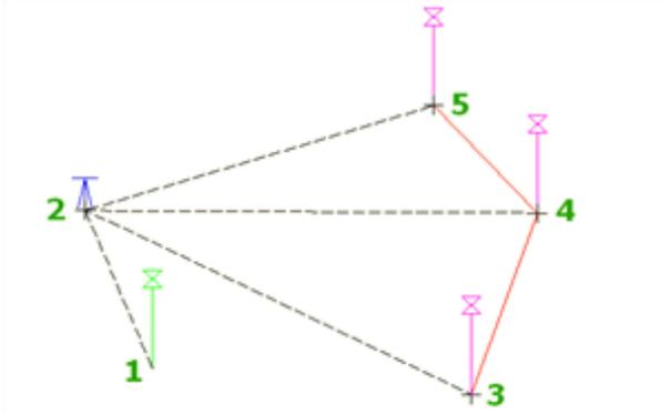
To define a line, you can either select an existing line in the drawing or enter two points. If you have already entered one point in the command, you are prompted to enter a second point to define the reference line.
