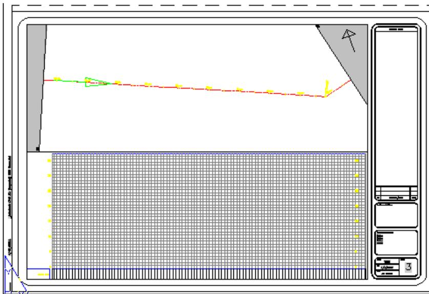
The Display tab of the Match Line Style dialog box includes an option to specify a hatch pattern for this match line mask area. Use this option to help you make your construction documents look better by masking the drawing data that exists outside of the match lines. See [Editing the Match Line Mask Area](#) (page 1923) for more information.
