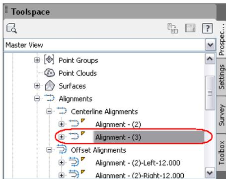
The Explore In Prospector command is available for centerline alignments, offset alignments, and curb return alignments, and is available from the Intersecting Alignments collection as well as from the Intersection Quadrants collection.
