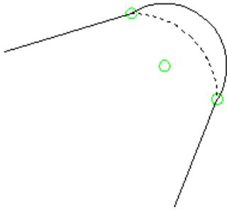
If the curve is not tangent, the Maintain Tangency button is activated. If you toggle this button the curve will be adjusted to make it tangent to the adjacent segments. If the curve is tangent, the button is disabled.
