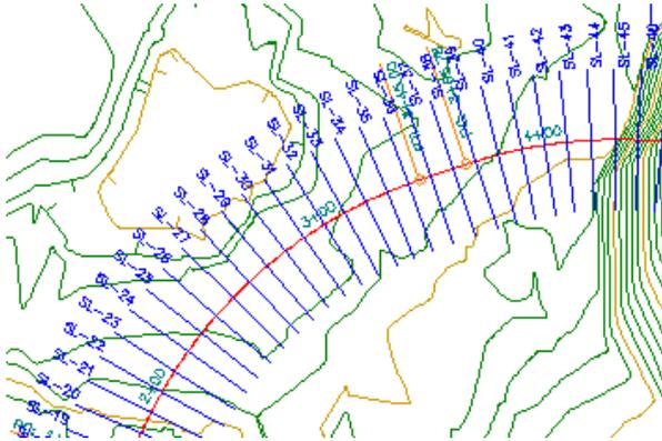
Sample lines are linear objects that are used to cut sections across an alignment. Sample lines have their own styles and can be labeled (for example, SL-29). A set of sample lines makes up a named collection called a sample line group. A sample line group centrally manages the display styles and label styles for a number of sample lines, sections, section views, and mass haul lines and mass haul views.
