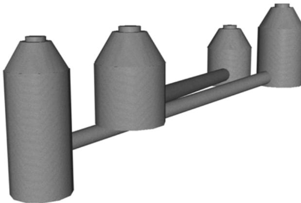
You can run an interference check that identifies parts in their 3D representation that are less than a specified distance away from any part in the other network. The distance is checked in every direction surrounding each part.
