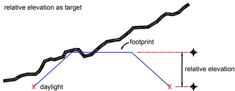
Section view of relative elevation as target
