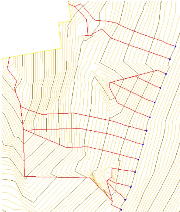
You can use either a 2D or 3D polyline to draw the flow line. The line type that you use depends on your analysis requirements. Following are usage examples for each line type:
