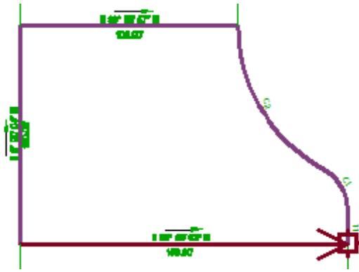
In the Survey Command Window you have the option to list mapcheck information that computes the error of closure for a figure based on the precision settings for direction and distance values which you specify in the [Survey Database settings](#) (page 2698) For more information, see [Listing Mapcheck Information for a Figure](#) (page 384).
