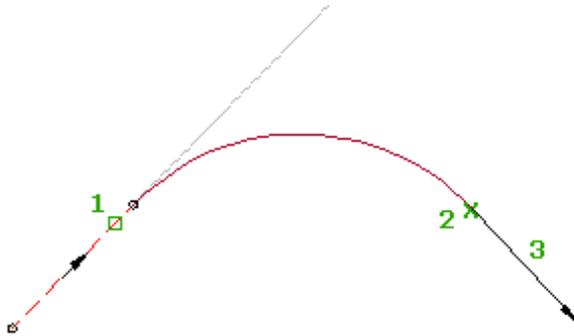
The result is a floating curve that is always tangent to the entity it is attached to.
