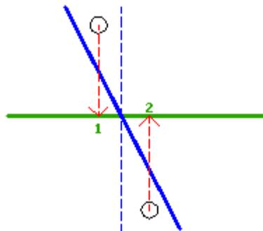
In cases where you have non-perpendicular or non-radial sample lines, an object that appears to be “before” or “after” a sample line can actually be in the opposite position because of the way the object’s station is determined relative to the alignment.
