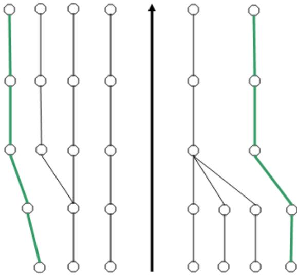
Outward branching and extra points (with the same point code) are not connected:
