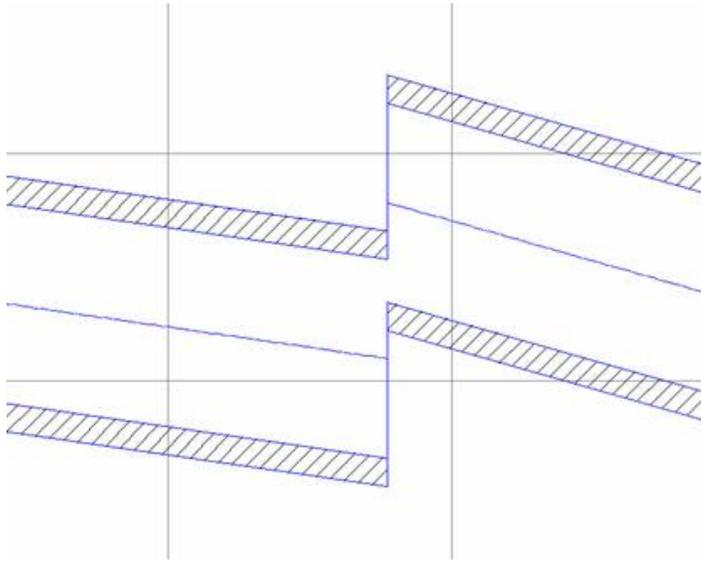
When this option is not checked, the appearance of pipe to pipe connections displayed in profile view is not cleaned up. The following illustration shows a profile of a pipe to pipe connection with the pipe end clean up option turned off.
