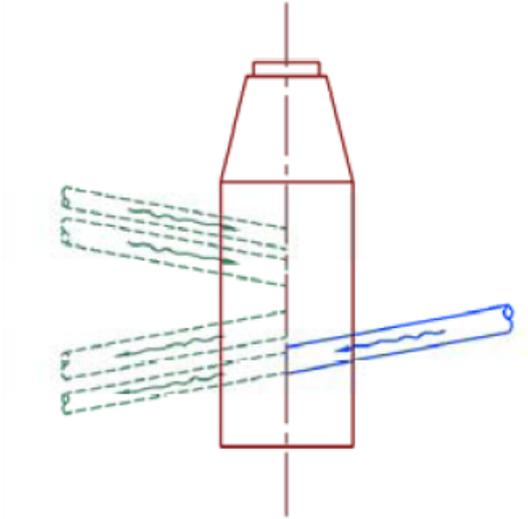
The following illustration shows a similar situation with both incoming and outgoing pipes already connected. In this case, a new *outgoing* pipe is added to the structure. The pipe cover and slope rule determines the optimal connection elevation for the new outgoing pipe.
