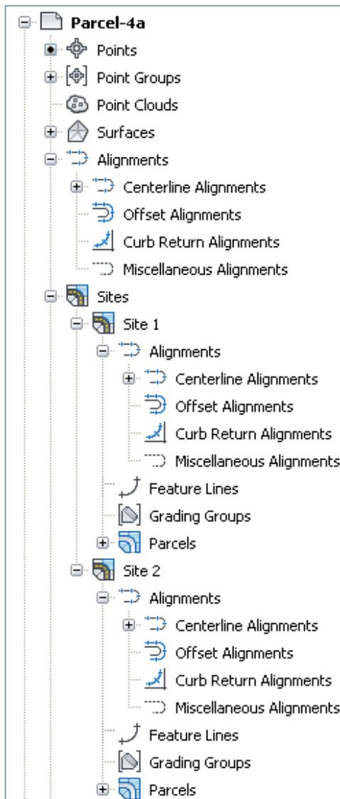
If you do not want an alignment to interact with other objects, accept the default <None> site selection when you create the alignment. Alignments can be moved or copied onto sites at a later time if interaction with other objects is desired.
