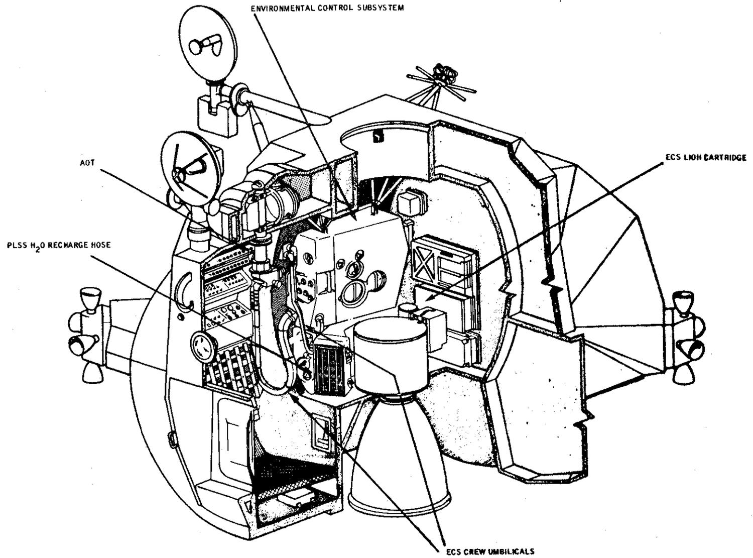
Cutaway of LM cabin interior, left half
