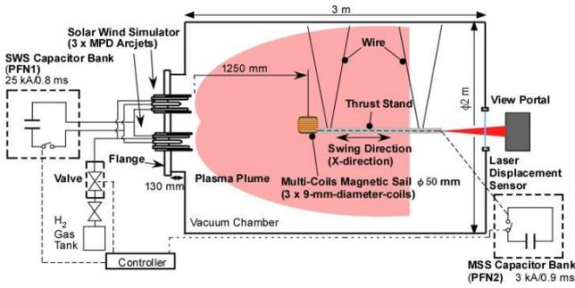
Fig. 3. Experimental configuration of Multi-Coil Magnetic Sail.
