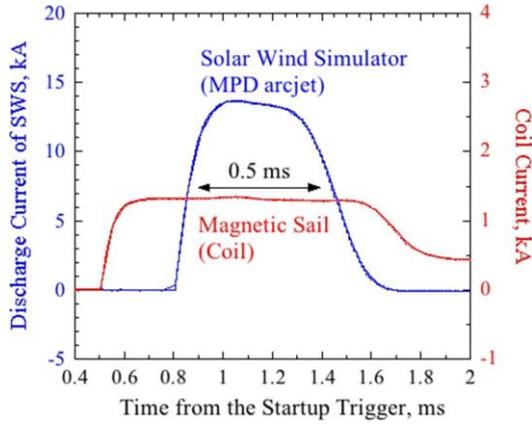
Fig. 4. Profiles of the current of SWS (charging voltage = 2.7 kV) and the coil current (charging voltage = 1.5 kV).
