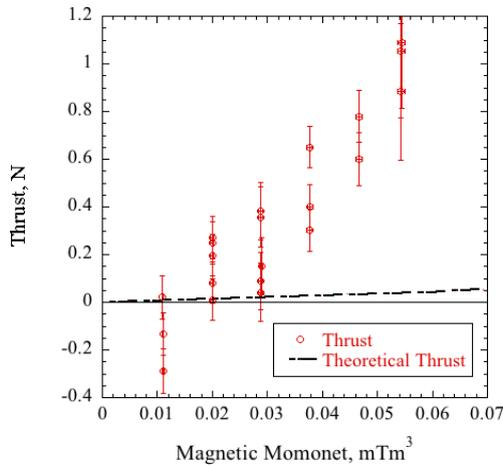
Fig. 6. Thrusts of multi-coil magnetic sail for various magnetic moments (SWS charging voltage = 2.7 kV).
