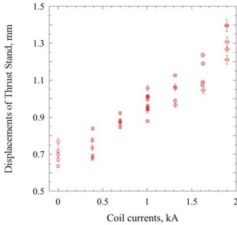
Fig. 5. Measured displacements of thrust stand for various coil currents (SWS charging voltage = 2.7 kV).
