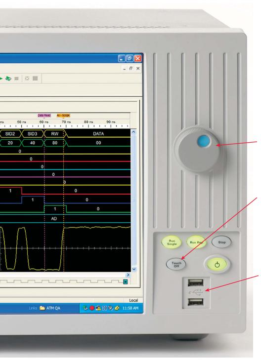
General-purpose knob lets you quickly adjust your viewing and measurement parameters. Select a modifiable variable, then turn the knob to quickly step through values for the variable.
