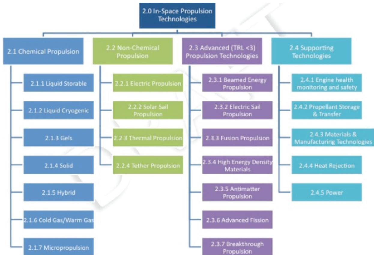
**Figure 1.** *In-Space Propulsion Technology Area Breakdown Structure*
