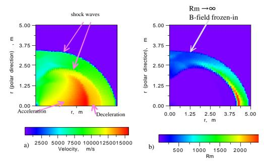
Fig. 7 Evolution of plasma; a) velocity distribution, b) magnetic reynolds number distribution..
