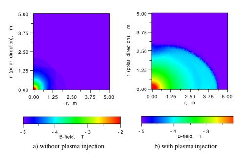
Fig.6 Inflation of magnetic field; magetic flux density distribution at t=0.22ms after plasma injection; logarithmic scale.
