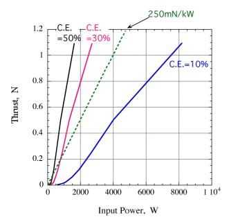
Fig. 3 Thrust to power ratio of magnetoplasma sail obtained from the electric power required to expaned the magnetic field.
