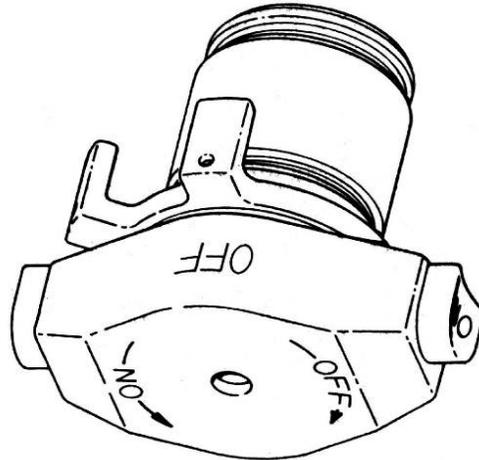
Figure 27 The Pressure Control Valve (PCV) (Courtesy K. Thomas)
