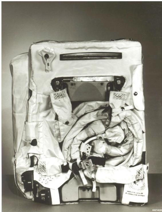
Figure 43 The Apollo 15-17 PLSS (Courtesy United Technologies Aerospace Systems)
