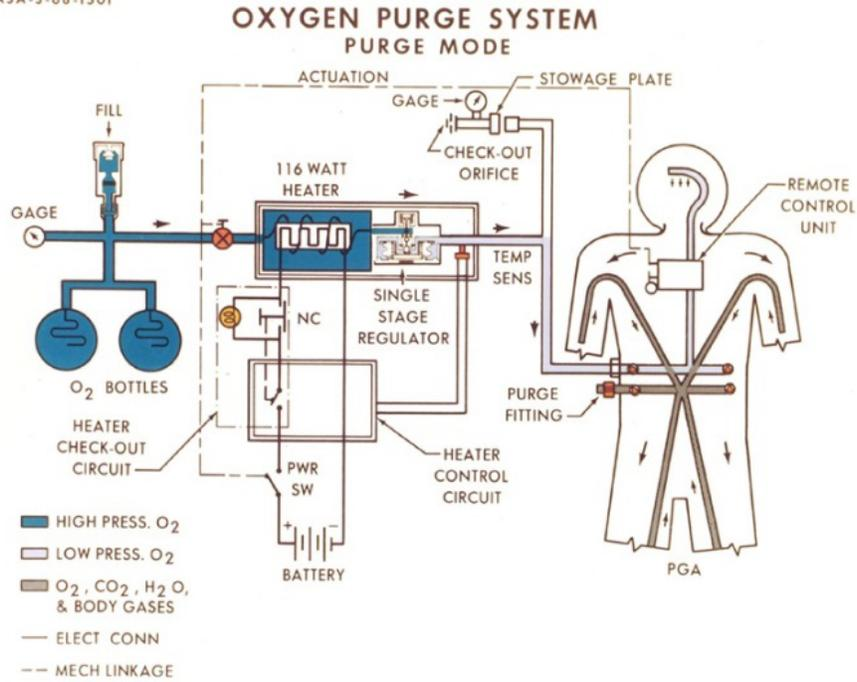
Figure 21 The Apollo 9-14 Oxygen Purge System (Courtesy NASA)
