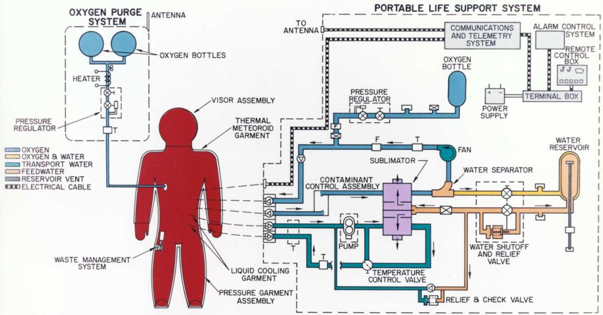
Figure 24 The Apollo 9 to 14 EMU Schematic (Courtesy NASA)
