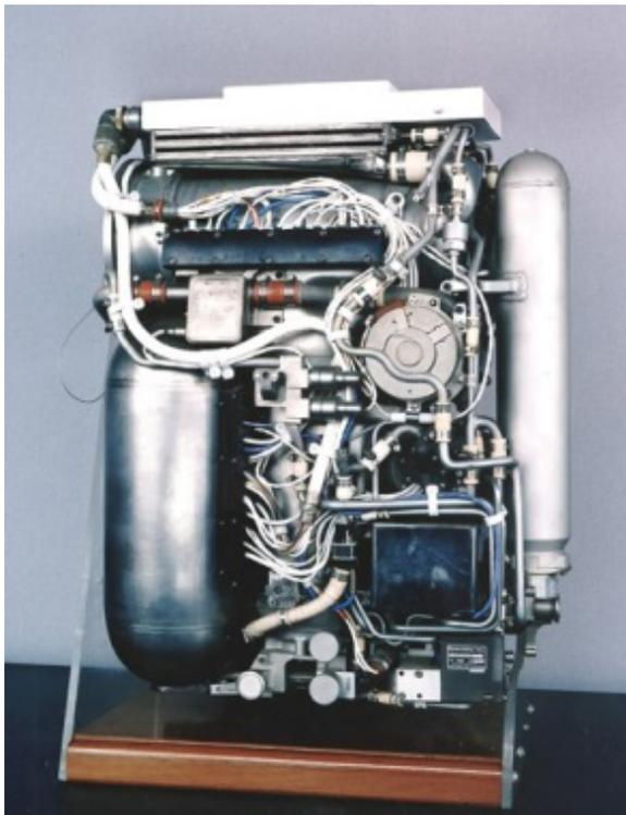
Figure 42 The Apollo 15-17 PLSS (Courtesy United Technologies Aerospace Systems)
