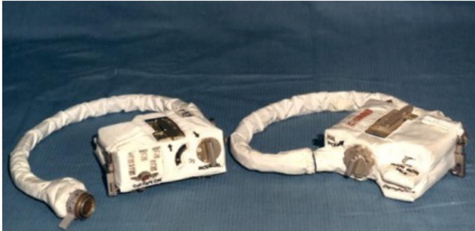
Figure 31 The Apollo 11-17 RCU (Courtesy United Technologies Aerospace Systems)
