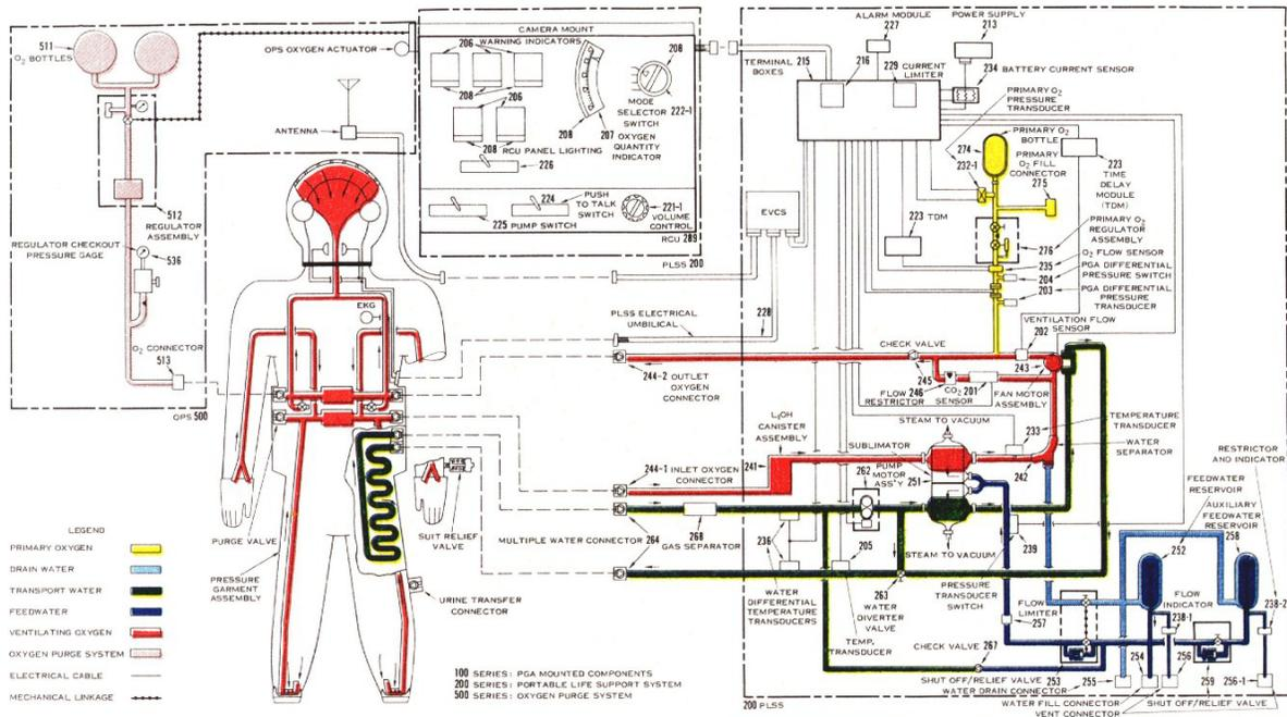
Figure 41 The Apollo 15-17 PLSS (Courtesy United Technologies Aerospace Systems)
