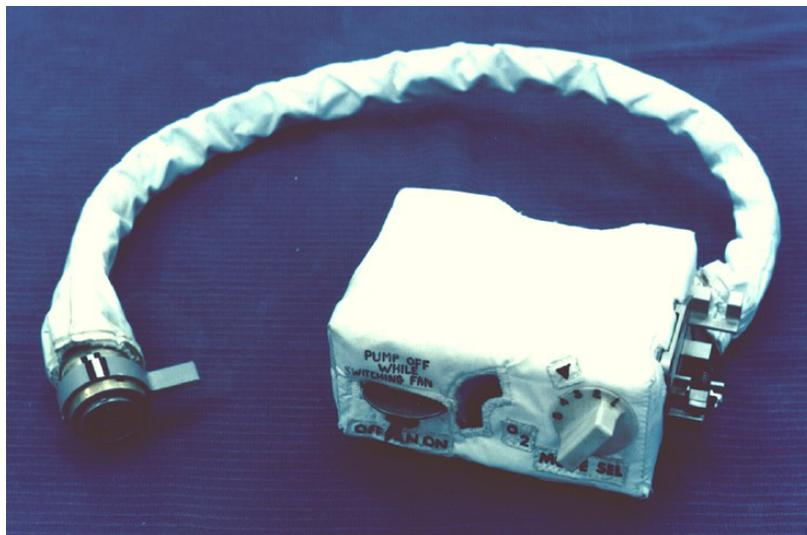
Figure 23 The Apollo 9 and 10 Type RCU (Courtesy United Technologies Aerospace Systems)
