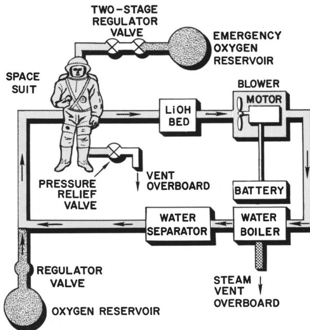
Figure 5 The First Apollo PLSS Schematic
