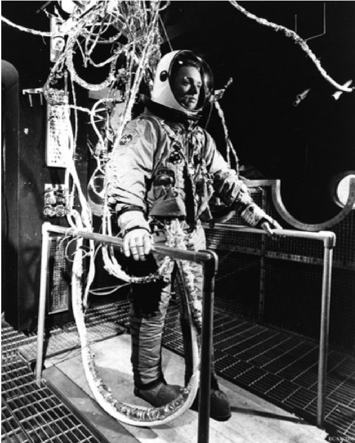
Figure 17 1965 Successful Apollo EMU Chamber Testing
