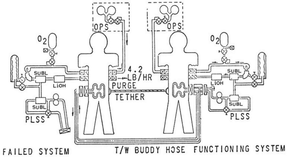
Figure 38 The BLSS System Schematic (Courtesy K. Thomas)
