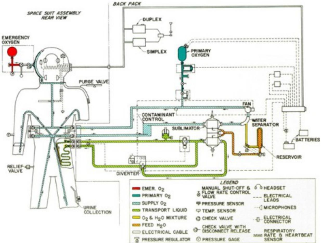
Figure 16 The -1 (Dash One) Liquid-Cooled PLSS Schematic
