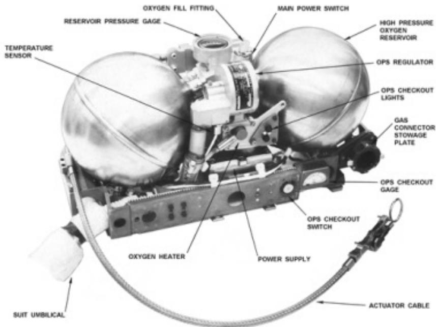
Figure 20 Oxygen Purge System (OPS) Components (Courtesy United Technologies Aerospace Systems)
