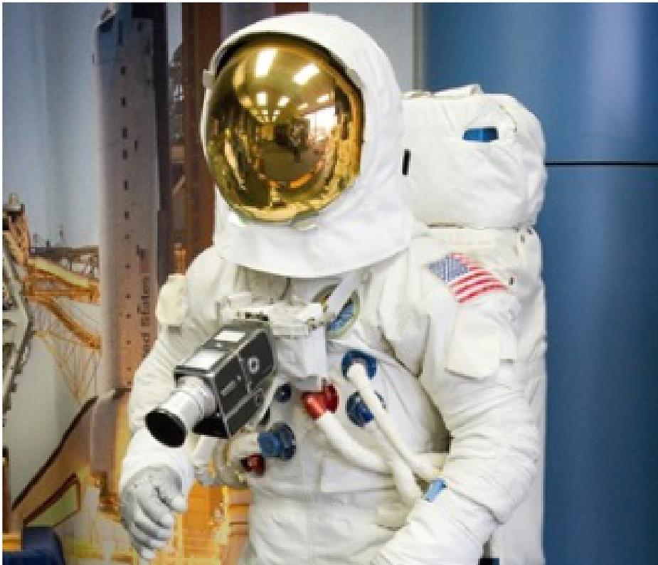
Figure 32 Camera and Bracket Attached To The RCU (Courtesy United Technologies Aerospace Systems)
