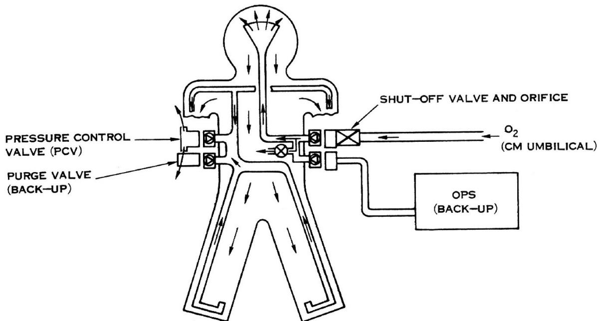
Figure 28 EMU Schematic Using PCV (Courtesy K. Thomas)
