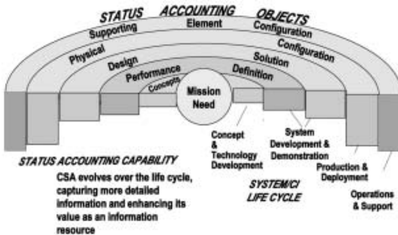
Figure 6. Configuration Status Accounting Evolution over the System/CI Life Cycle
