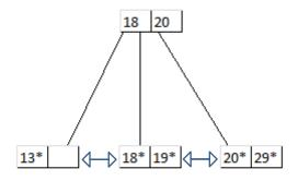
Insert 27: No room for 27. Between 20-27-29, 27 moves to upper node. Between 18-20-27, 20 moves to the upper node:
