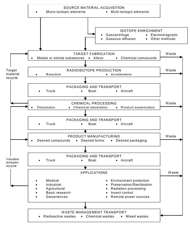
**FIGURE 1.** Flow of radioisotope production, manufacturing, applications, and waste management
