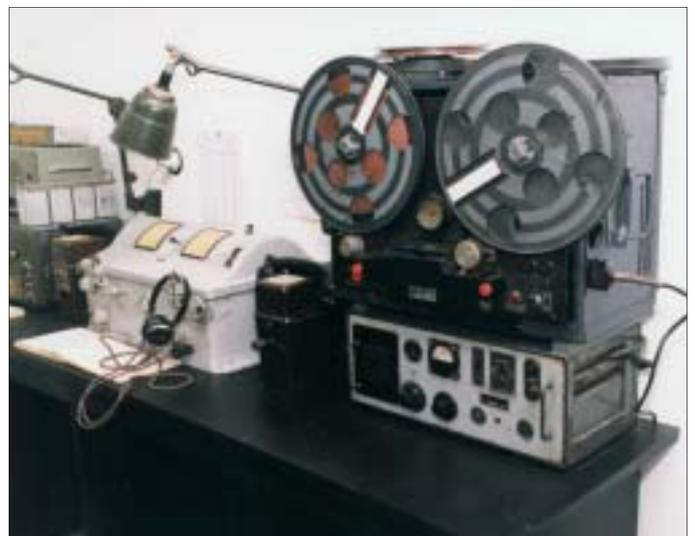
To receive and record news emitted by illegal transmitters, a short band receiver Spez.860 Bs. and tape recorder AEG, model Ton. S.b. were used.
